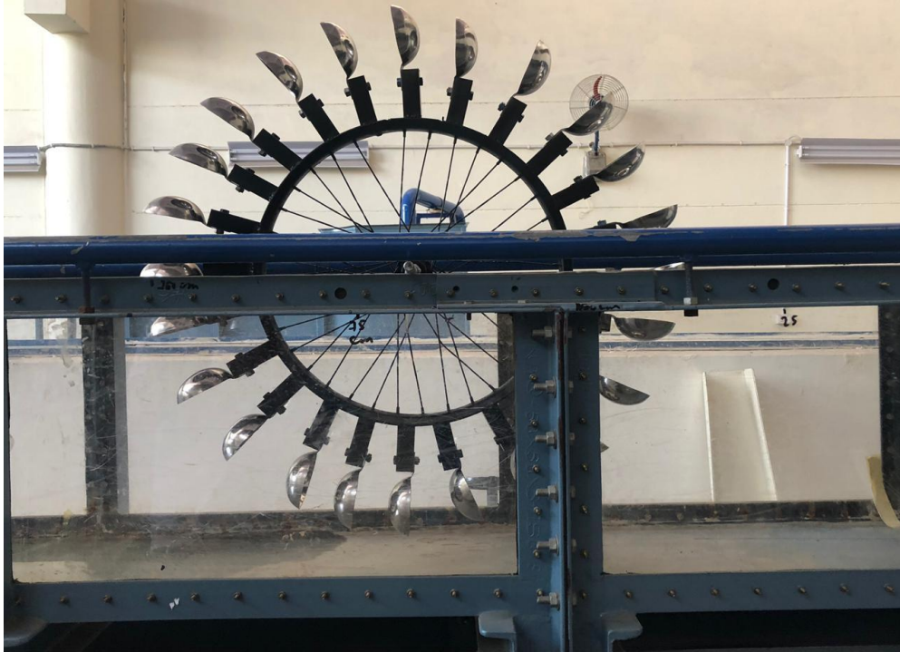
Fig. 3.3: Actual image of Hydraulic wheel designed for the flume.
