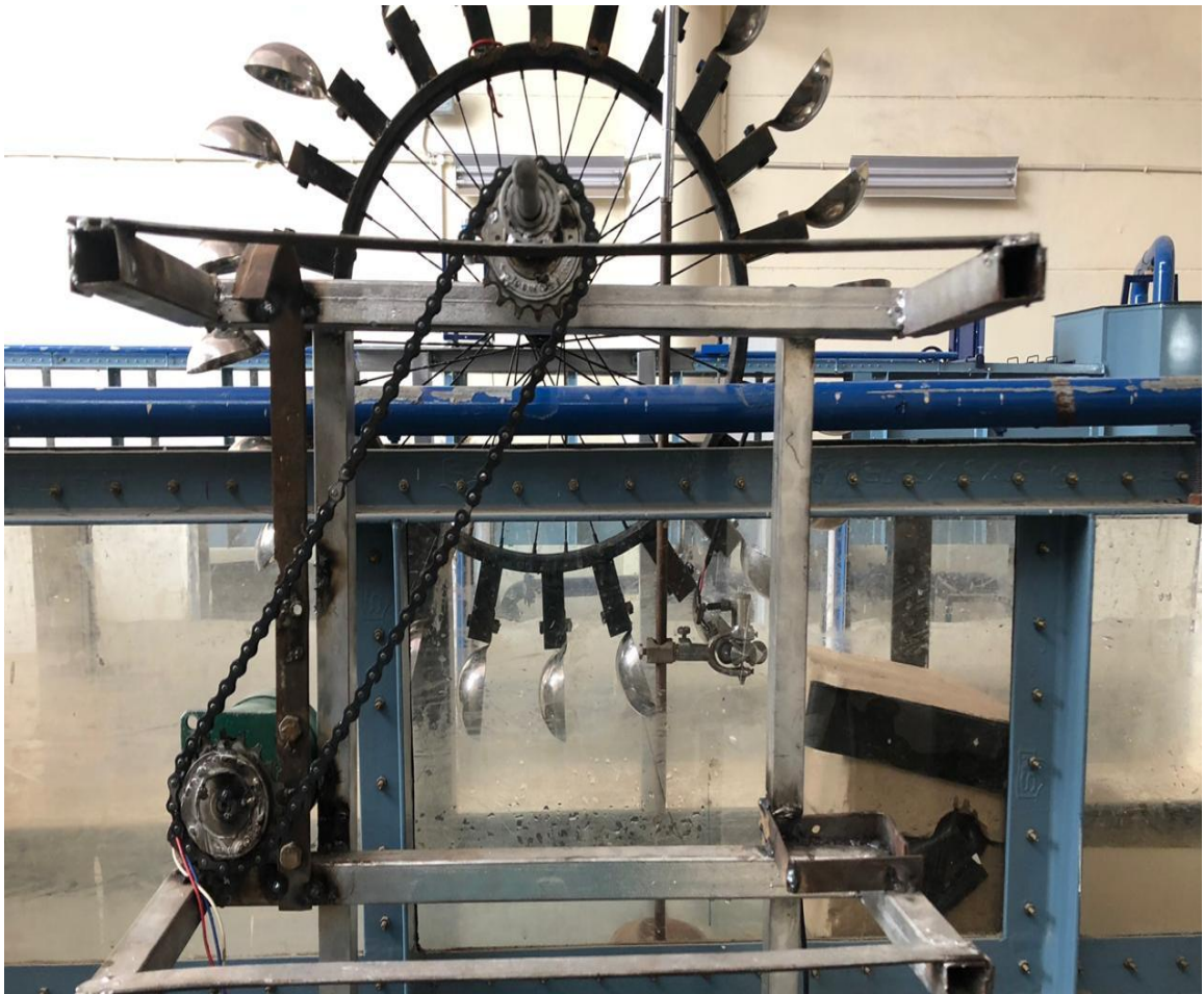
Fig. 3.8: Image showing the gear chain mechanism used for transmission of mechanical energy to the DC Generator.
