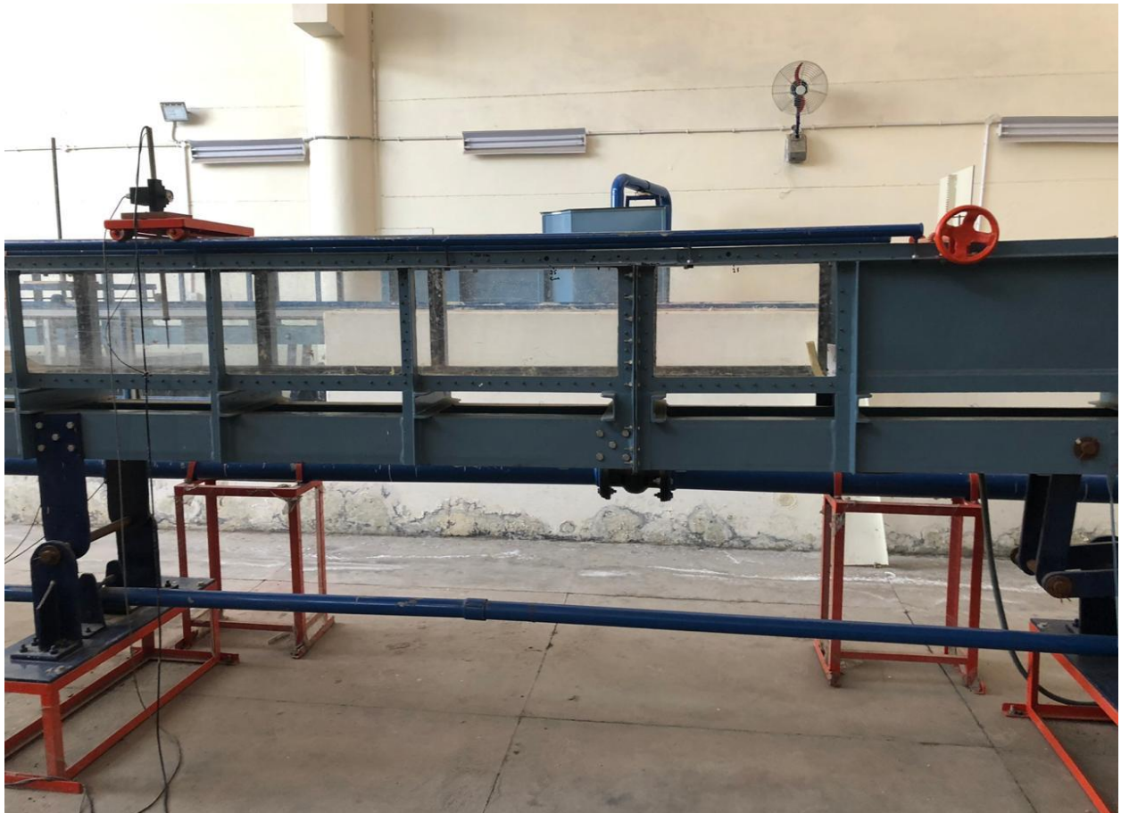
Fig.3.1: Flume used for testing the model for different flow rates.
