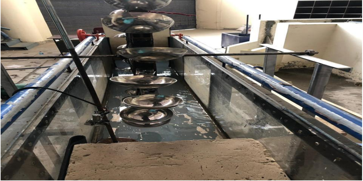
Fig. 3.5: Image showing Spoons used as blades of the flywheel.
