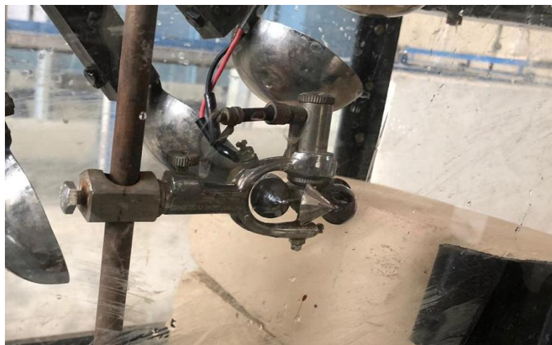
Fig.4.4: Rotating current meter which is connected to the above digital velocity meter.
