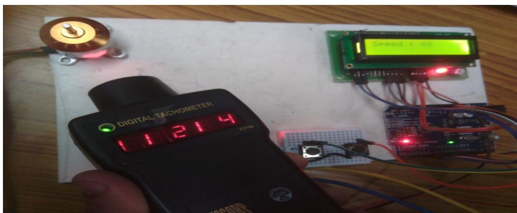
Fig5.37 Speed for 80% duty cycle, 11214 rpm
