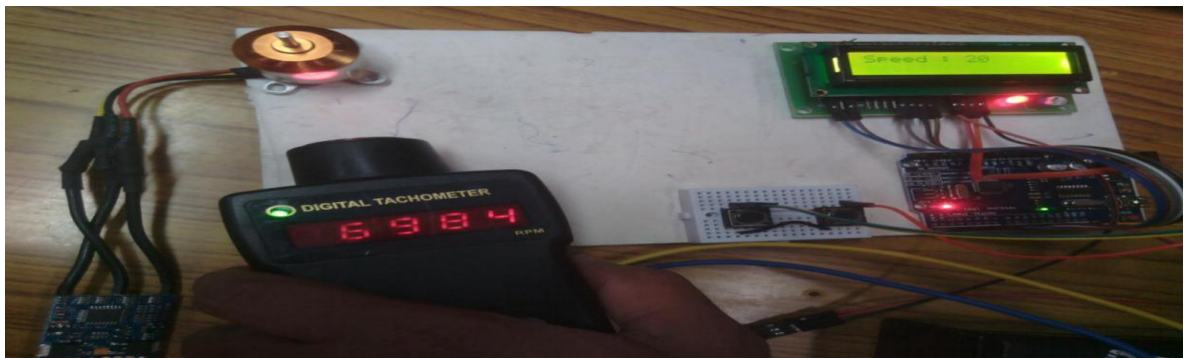
Fig5.19 Speed for 20% duty cycle, 6984 rpm
