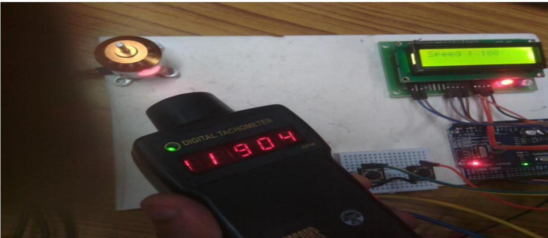
Fig5.43 Speed for 100% duty cycle, 11904 rpm
