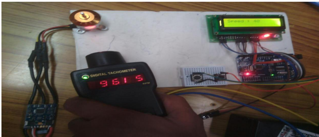
Fig5.25 Speed for 40% duty cycle, 9615 rpm
