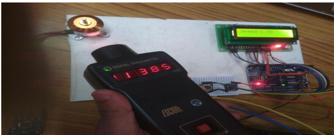
Fig 5.40 Speed for 90% duty cycle, 11385 rpm
