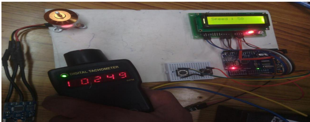
Fig5.28 Speed for 50% duty cycle, 10249 rpm
