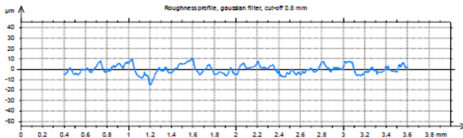
Figure 15.06: R_a=2.59 mm profile of AL6061+SiC composite
