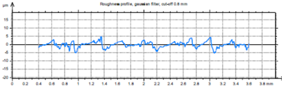
Figure 15.20: R_a=1.62\text{mm} profile of AL6061+SiC composite
