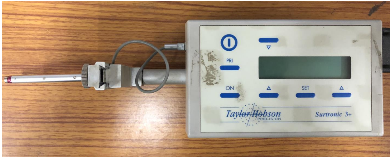
Figure 1.2: Surface roughness measurement apparatus in Metrology Lab
