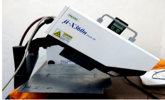
Figure 4.4: Experimental set-up for residual stress measurement using portable X-ray machine ( \mu -X360) in Precision Lab
