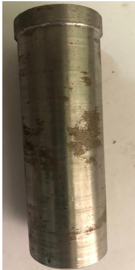
Figure 1.1: Work piece Material of AISI 8620 steel
