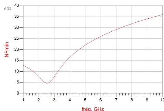
Fig. 8: Noise Figure of the LNA circuit with matching network 1
