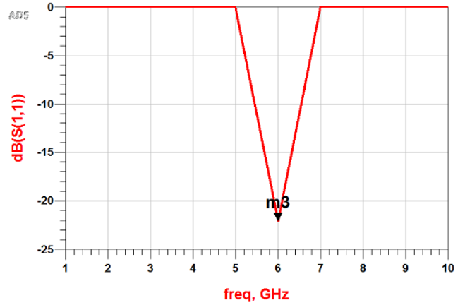
Fig. 3: Input Return Loss
