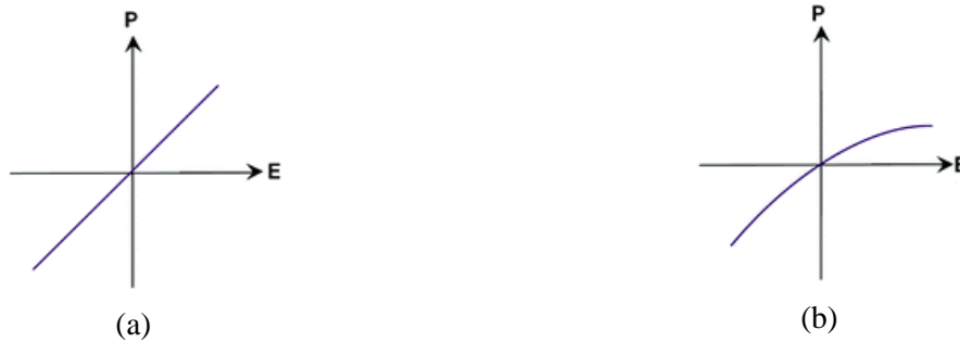
Figure 1.1: Relationship between the electric field E vector and polarization P vector (a) in a linear medium and (b) in a nonlinear medium [33].
