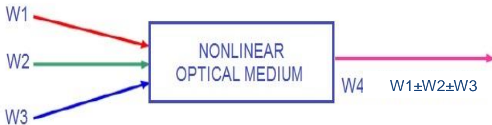
Figure 3.1: Basic mechanism of four wave mixing [39].
