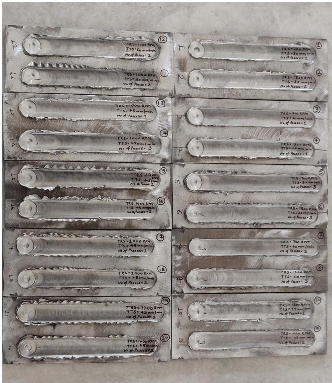
Figure 3.8: Grooves after the friction stir processing in advance metal joining lab
