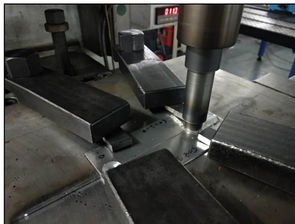
Figure 3.5 Friction Stir Welding of AA5083-O and AA6082-O
