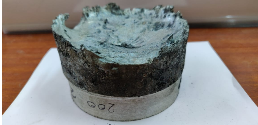
Figure 4-3 Casting of AMC with B4C MS 200
