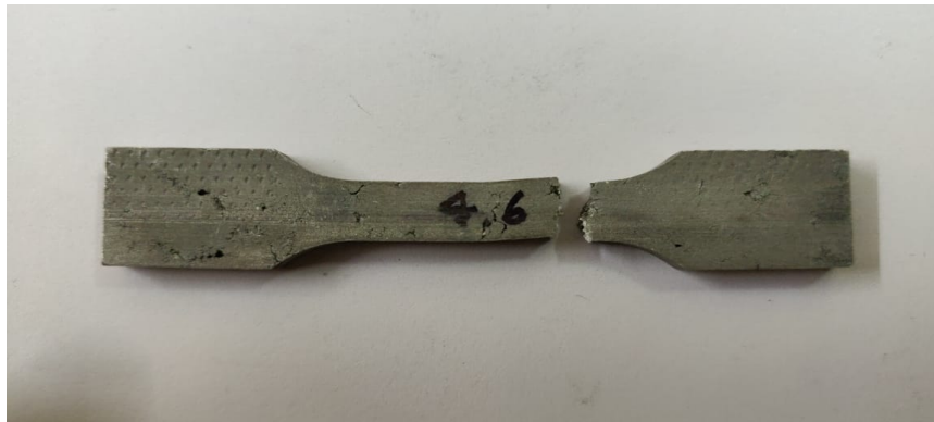
Figure 4-19 AMC MS 270 specimen after tensile test
