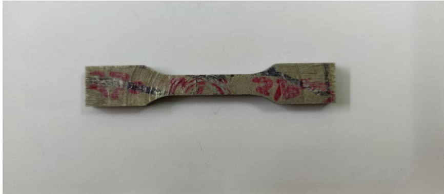
Figure 4-18 AMC MS 270 specimen before tensile test
