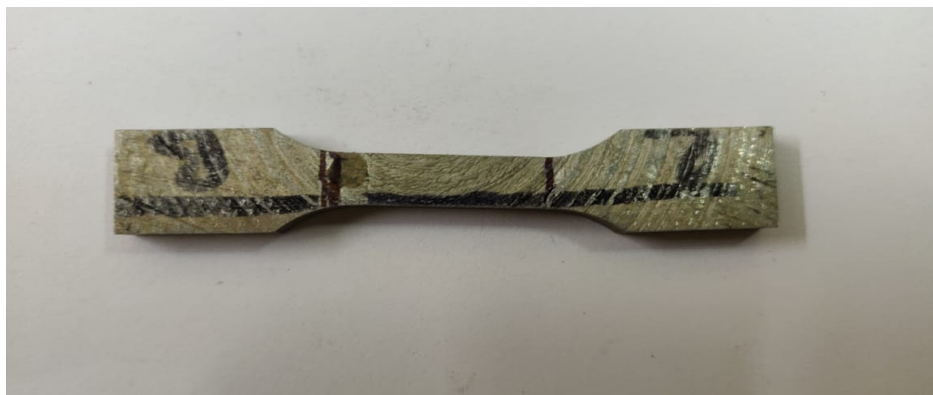
Figure 4-14AMC MS 150 specimen before tensile test
