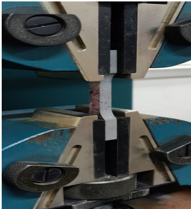
Figure 4-11 Closer view of specimen subjected to tensile loading
