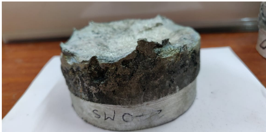
Figure 4-4 Casting of AMC with B4C MS 270
