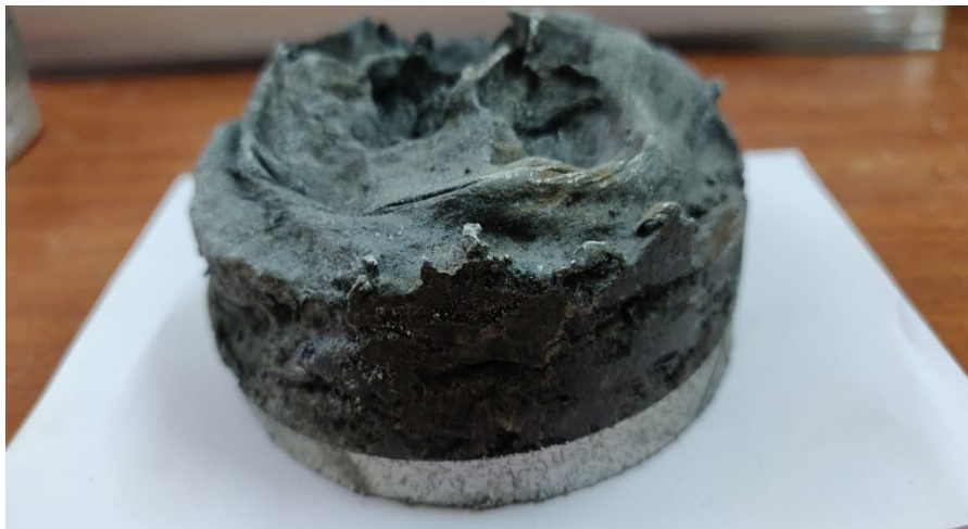
Figure 4-2 Casting of AMC with B4C MS 150
