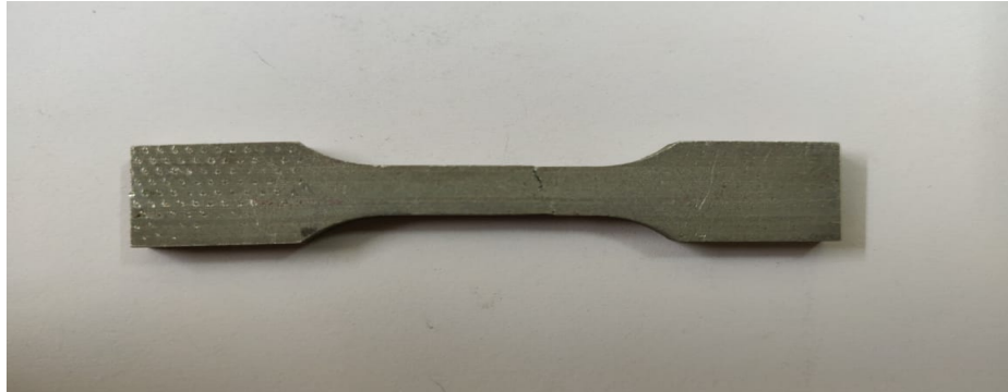
Figure 4-12Base alloy specimen before tensile test
