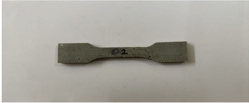
Figure 4-16 AMC MS 200 specimen before tensile test
