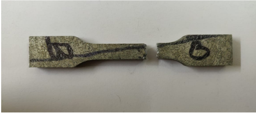
Figure 4-15 AMC MS 150 specimen after tensile test
