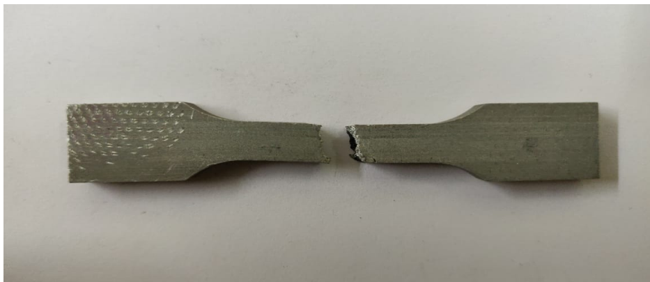
Figure 4-13Base alloy specimen after tensile test
