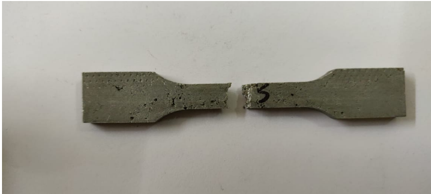
Figure 4-17 AMC MS 200 specimen after tensile test
