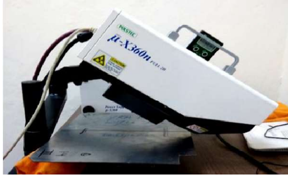
Figure 4-12 Experimental set-up for residual stress measurement using portable X-ray machine ( \mu -X360)
