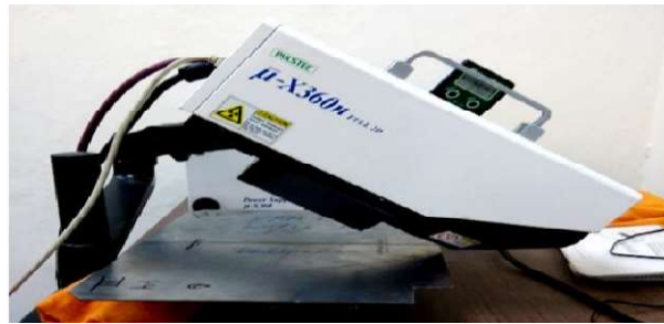
Figure 3-16 Experimental set-up for residual stress measurement using portable X-ray machine ( \mu -X360)
