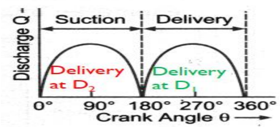
Figure 3 8: Double Acting Discharge Variation
