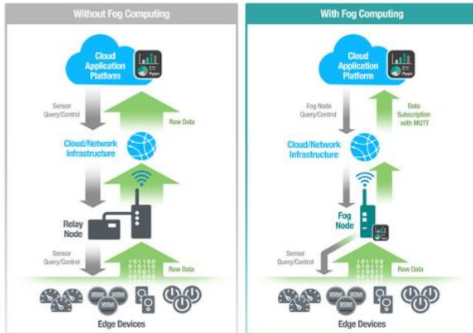
Figure6: Cloud Computing vs. Fog Computing
