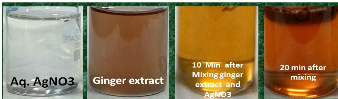
Fig:3.1. Change in colour after mixing of ginger extract and aq. AgNO 3 .
