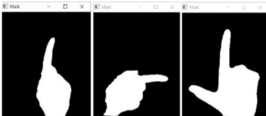
Figure 6 Segmented Image with skin detection
