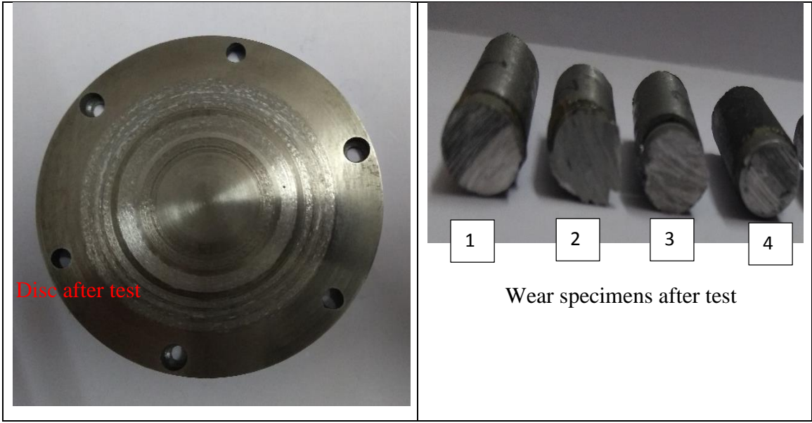
Figure 20 pin and disc after the wear test
