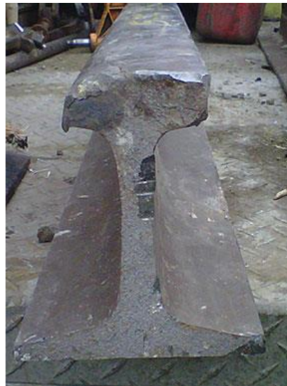
Fig.1.4: Plastic flow of metal from top surface to side face
