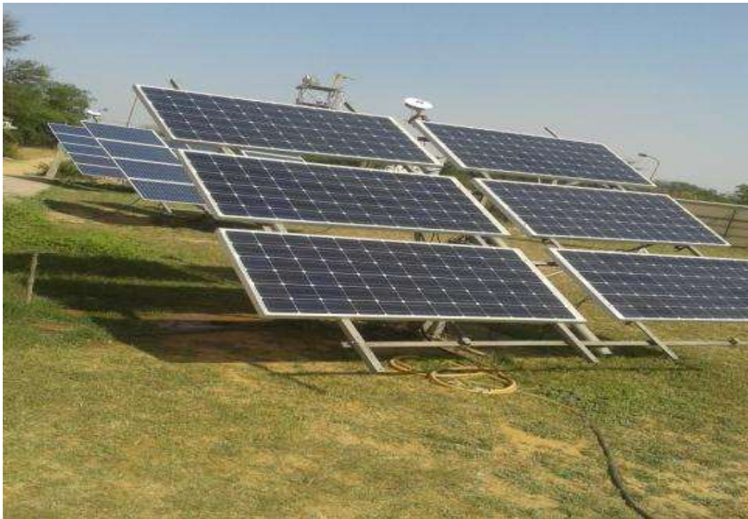
Fig. A.1 Experimental demonstration of Heterojunction with Intrinsic Thin Layer (HIT) solar PV module at National Institute of Solar Energy (NISE), India
