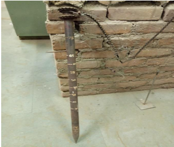
Fig 3.4 pile with a diameter 30mm
