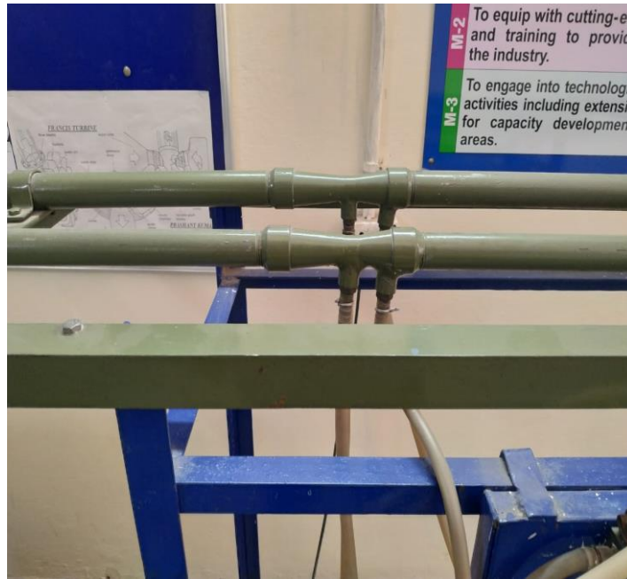
Figure 3.5 Laboratory arrangement for the two Venturi meters
