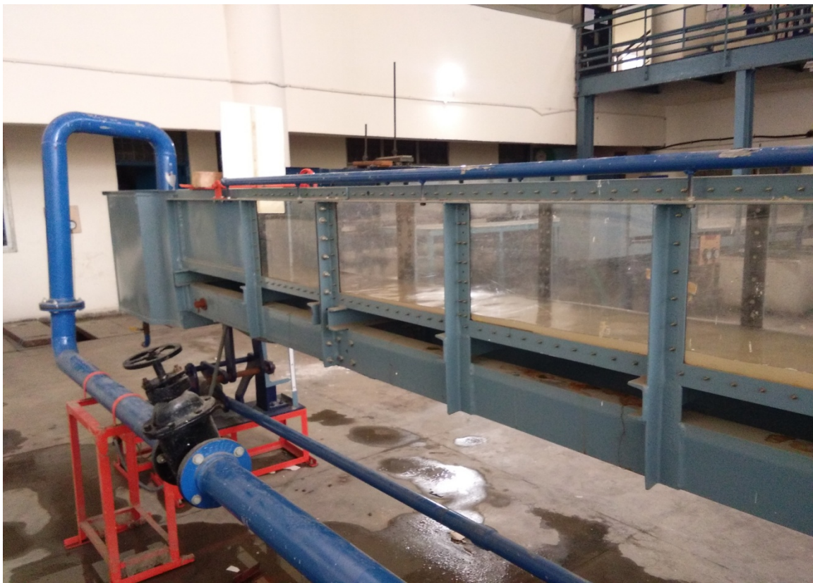
Figure 4.1 Inlet of the tilting flume
