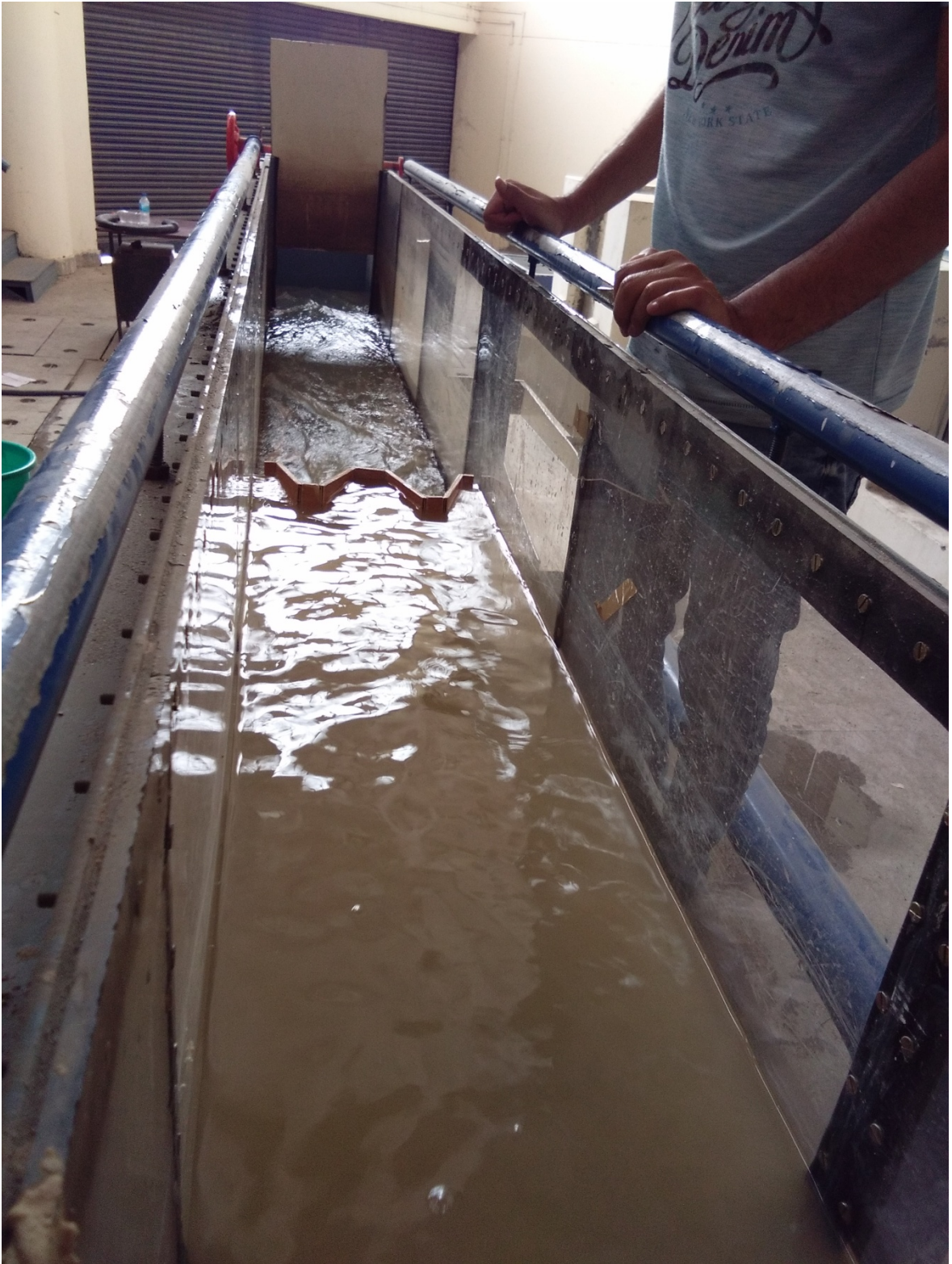
Figure 4.5 Placement of Weir in the Rectangular Flume
