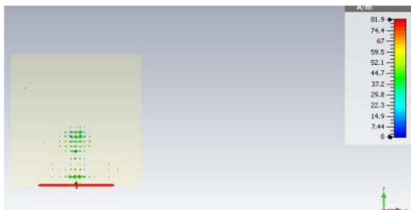
Fig. 6.6 Surface Current distribution at 8.8 GHz
