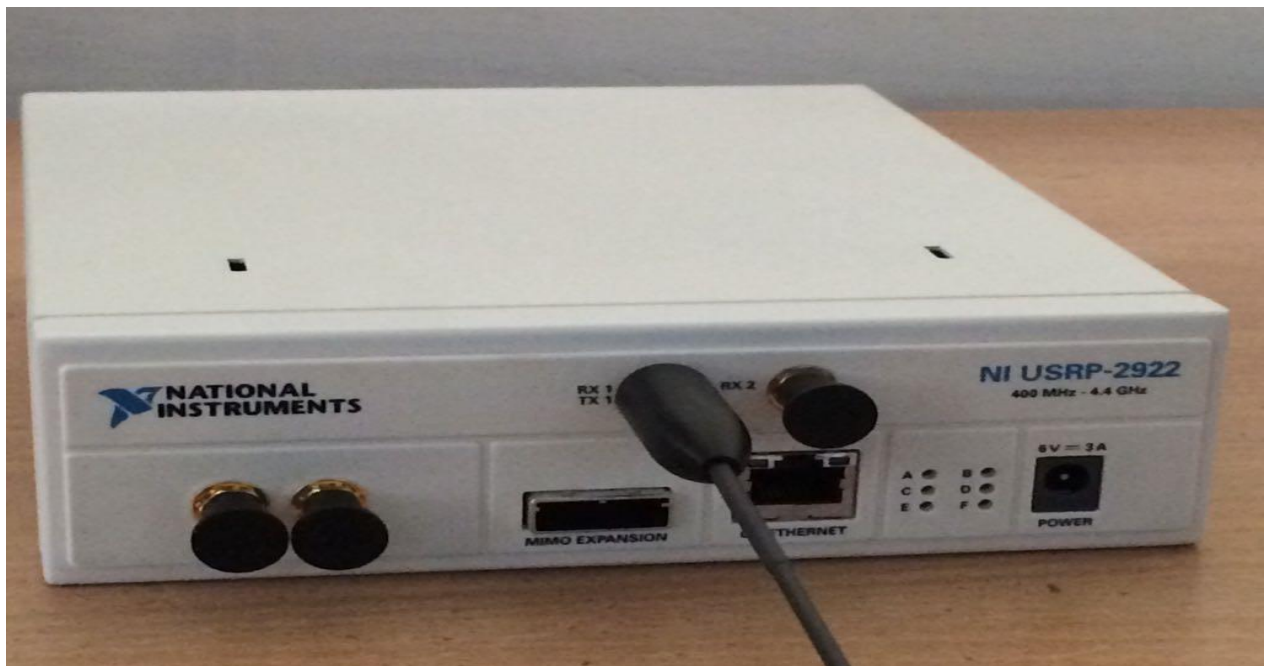
Figure 4.20: Power connections to the USRP kit
