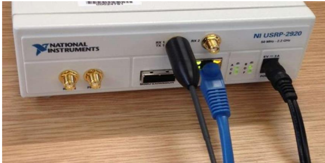
Figure 4.21: Ethernet cable and antenna connections to the USRP kit
