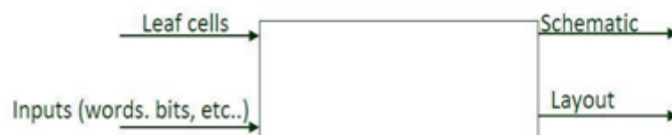
Figure 3.13 Function of Memory Compiler
