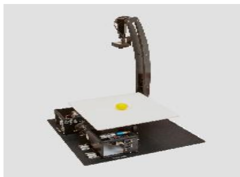
Fig :1 General structure of ball and plate balancer
