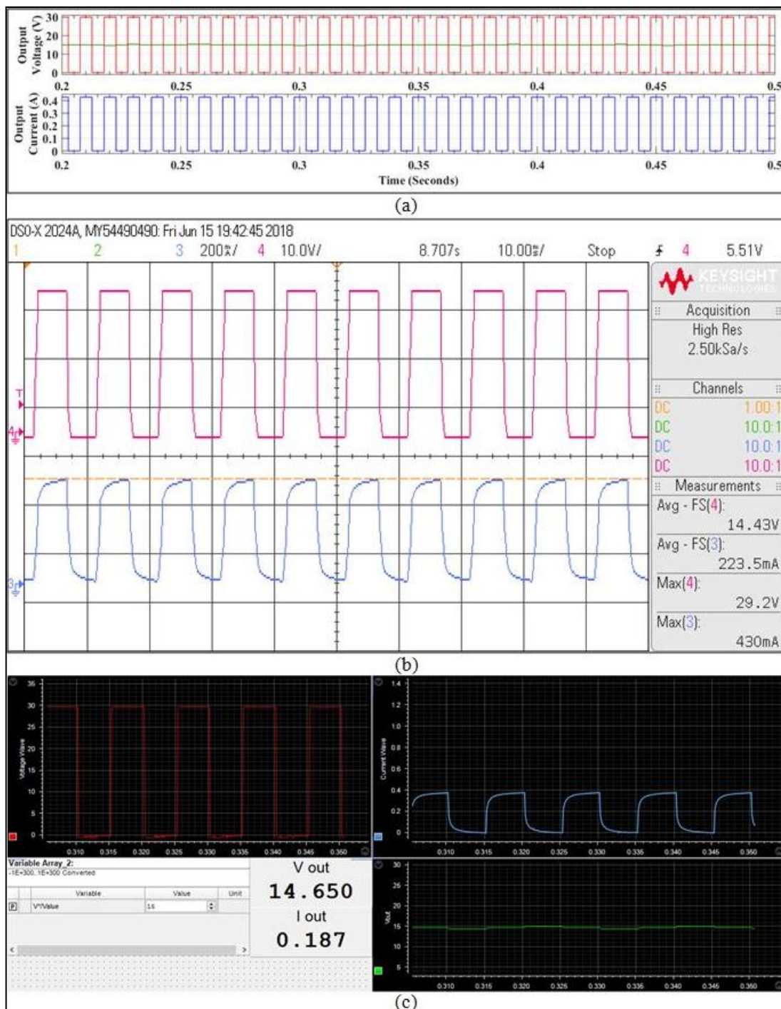
Figure 6.1: Voltage and current output of Open Loop Class-A Chopper at 50% duty cycle for R load:- (a) Output of Schematic in MATLAB Simulink; (b) Output of Hardware at DSO; (c) Output of Hardware in ControlDesk Software
