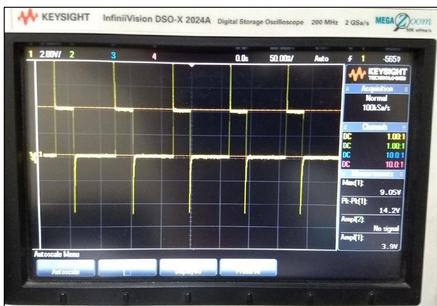
Figure A1.2: Voltage and current output of Chopper hardware with biasing problem
