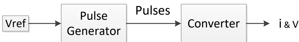
Figure 5.3: Block Diagram for Open Loop Configuration of Converter
