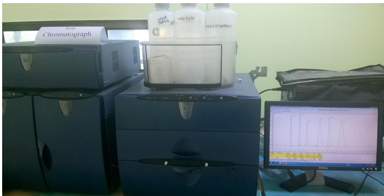
Figure 3.8 DIONEX-ICS-5000, USA (Cation and Anion Analyzer)
