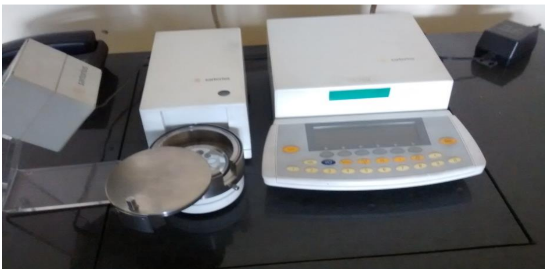
Figure 3.5 Sartorius microbalance used for weighing PM 10 and PM 2.5 Filter Paper
