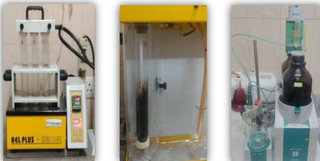
Figure 6.1: Kjeldahl apparatus: Digestion, distillation and titration (Kelplus Model KES06 L)
