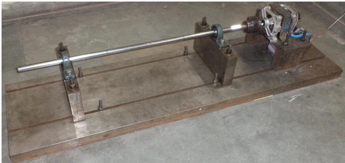
Figure 5.2: Actual rotor system for dynamic analysis
