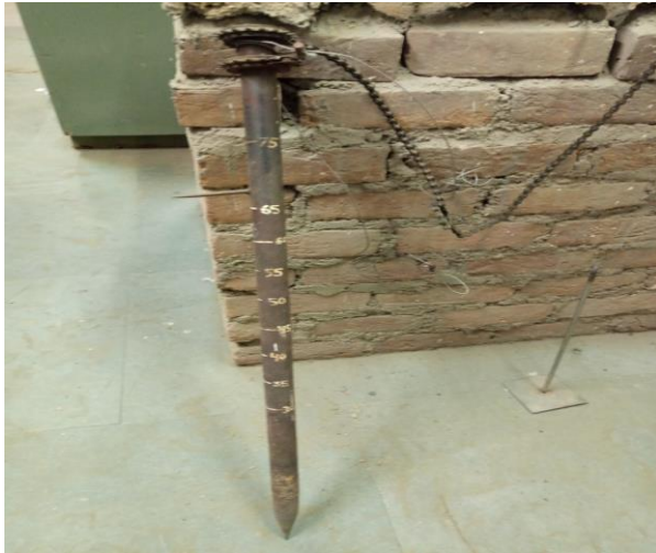
Fig 3.4 pile with a diameter 30mm
