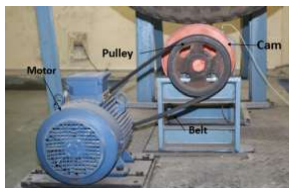
Figure 5.4: Road input arrangement
