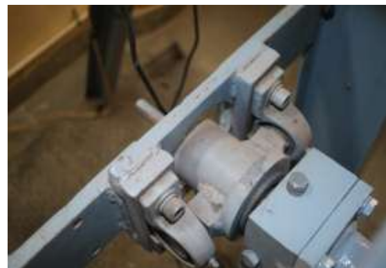
Figure 5.8: Special bearing arrangement for making hinge at one end of axle
