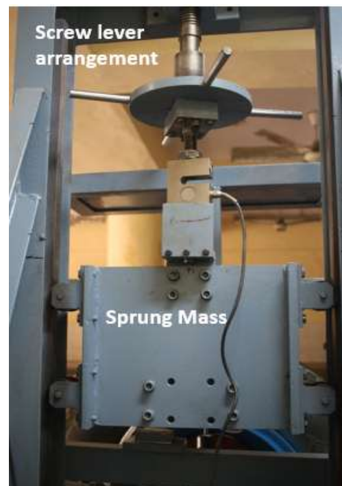
Figure 5.6: Screw lever arrangement for dead weight
