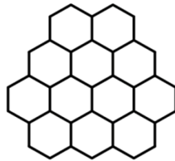
Fig.3.2: Structure of graphene
