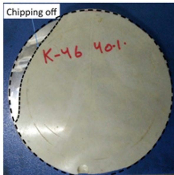
Fig.2.20: Post-blast visuals of SF46-40 syntactic foam after 5 repeated blast loadings ( P_r \sim 90 psi)
