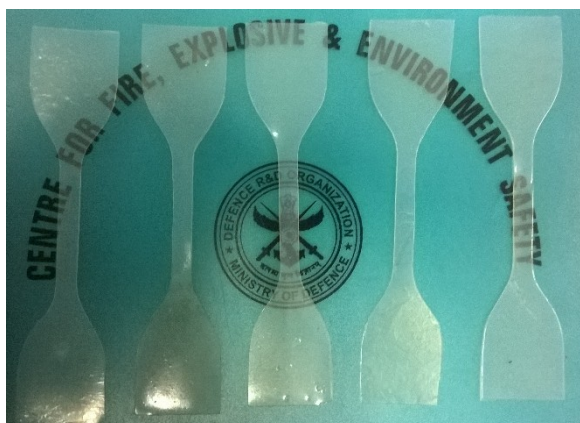
Figure 2.1: Transparent tensile coupons of polyurea (PU 230)
