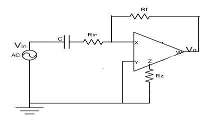
Fig 3.5 Circuit Diagram of First Order High Pass Filter
