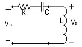
Fig. 4.17 Circuit Diagram of High pass filter
