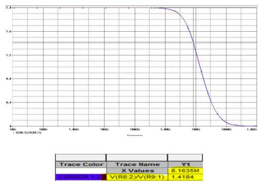
Fig 2.6 Frequency response of inverting amplifier with case 3
