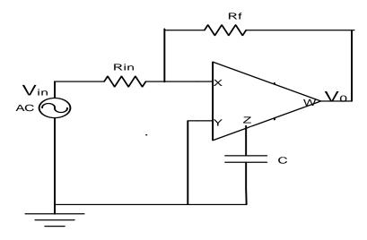
Fig 3.1 Circuit Diagram of First Order Low Pass Filter
