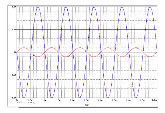
Fig. 3.4 Transient response of first order low pass filter
