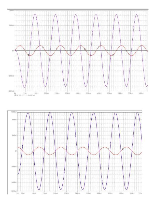
Fig 4.14 Transient response of Tow Thomas Biquad implementing band pass and low pass
