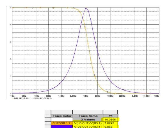
Fig. 4.12 Frequency response of Tow Thomas Biquad implementing band pass and low pass filter.
