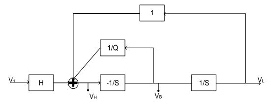
Fig. 4.10 Block diagram of Two Integrators in a Loop Biquad.[24]
