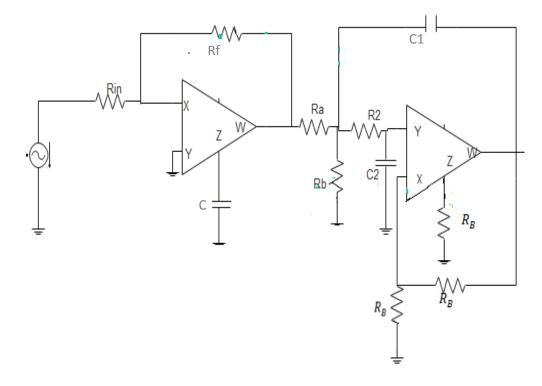
Fig 5.7 Circuit diagram of Chebyshev Third order low pass filter
