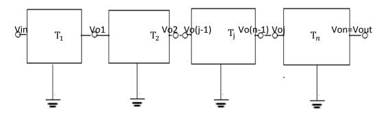
Fig 5.2 Cascade connections of Biquad sections to realize  $n^{th}$  order filter [11]
