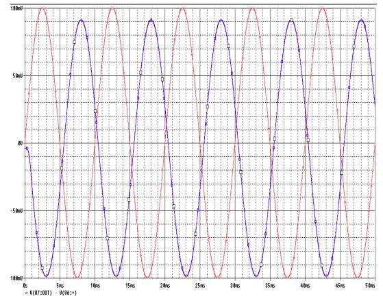
Fig. 5.5 Simulated Transient response of Butterworth fifth order low pass
