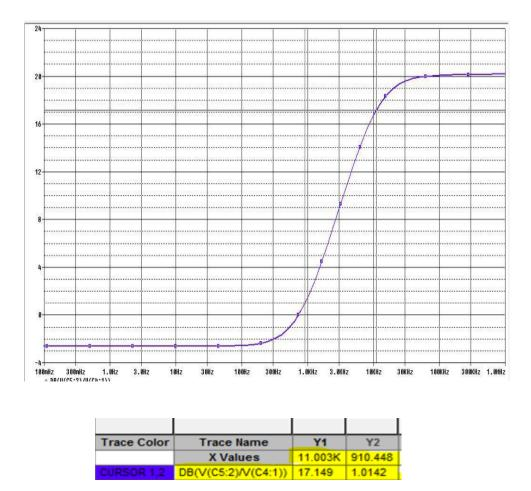
Fig 3.13 Frequency response of implemented bilinear transfer function
