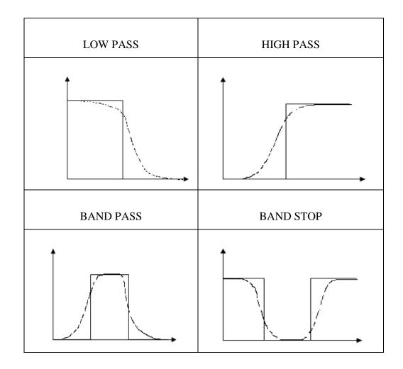
Table 1 Frequency Response of the Four Basic Filter Types. Ideal characteristics;Real characteristics.
