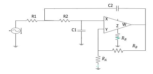
Fig. 4.3 Circuit diagram of SALLEN-KEY low pass filter According to the characteristics equation of the CFOA that is  $I_X = I_Z$  and  $I_Y = 0$ we can write the following equation
