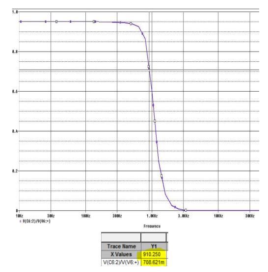
Fig 5.6 Simulated Frequency response of Butterworth fifth order low pass filter
