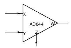
Fig 2.1 Functional Diagram of AD844 (CFOA)[14]
