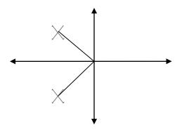
Fig 4.1 Pole locations of second order transfer function. For the maximally flat response Q should be equal to 0.707.
