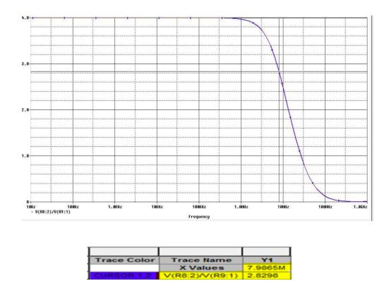
Fig 2.5 Frequency response of inverting amplifier with case 2
