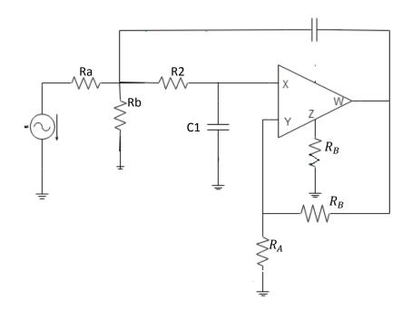
Fig 4.6 Circuit diagram of SALLEN-KEY low pass filter with gain adjustment
