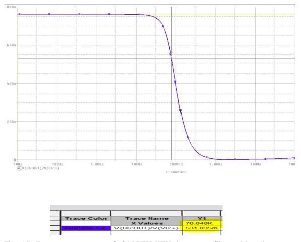
Fig 4.7 Frequency response of SALLEN-KEY low pass filter with gain adjustment
