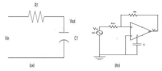
Fig 1.2 (a) Passive Low Pass filter and (b) Active low pass filter.
