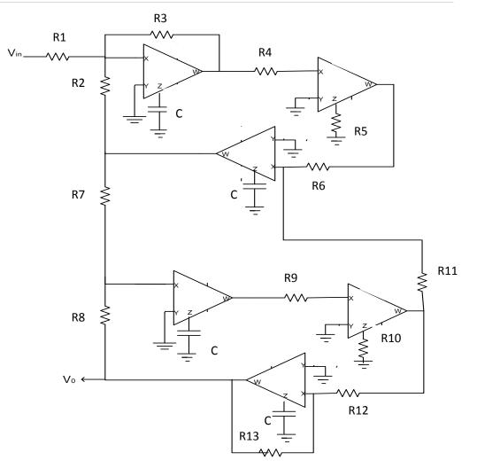
Fig 5.11 Active realizations of Low pass Ladder of Fig 5.8
