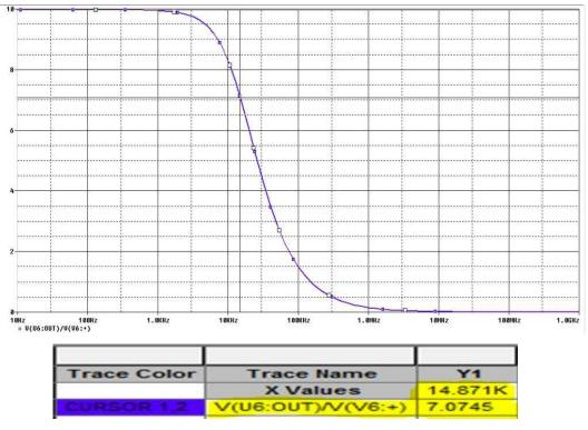
Fig 3.2 Simulated frequency response of first order low pass filter
