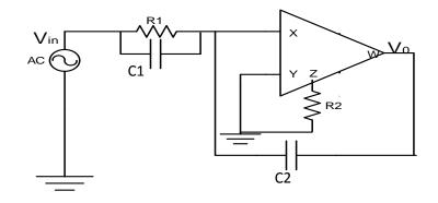
Fig 3.12 Circuit diagram implementing bilinear transfer function
