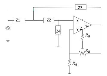
Fig 4.2 Circuit diagram of SALLEN-KEY configuration
