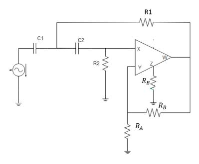
Fig. 4.8 Circuit diagram of SALLEN-KEY high pass filter
