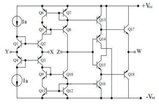
Fig 2.2 Internal Diagram of AD844 (CFOA)
