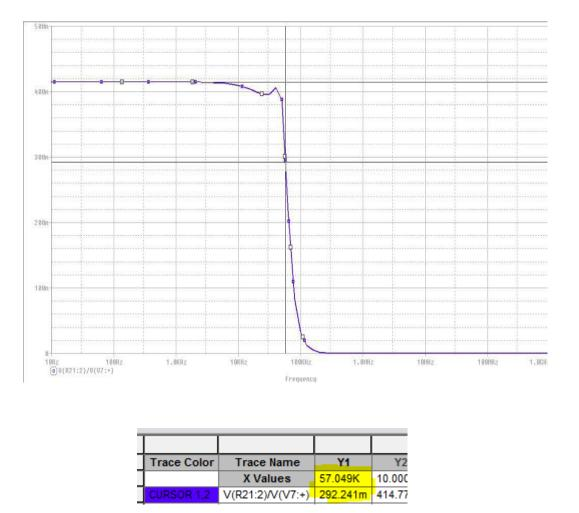
Fig 5.13 Simulating Frequency response of Fourth order LC low pass filter.
