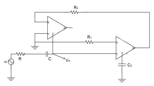
Fig. 4.19 Circuit diagram of high pass filter implemented using GIC.
