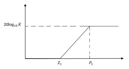
Fig 3.11 Ideal Characteristics of Bilinear Transfer Function with  $Z_1 > P_1$
