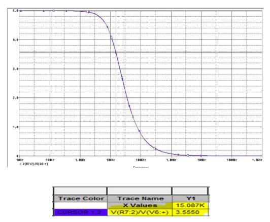
Fig 3.3 Simulated Frequency response of first order low pass filter with gain adjustment
