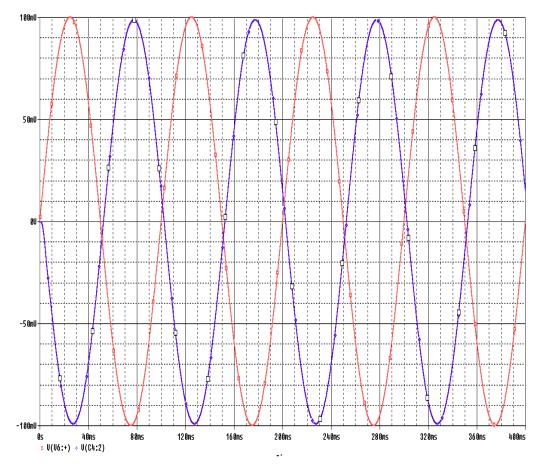
Fig 5.8 Simulated transient response of Chebyshev third order low pass filter
