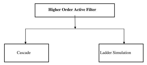
Fig 5.1 Approaches to design higher order active filter
