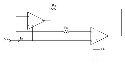
Fig. 4.15 Circuit diagram of grounded inductor
