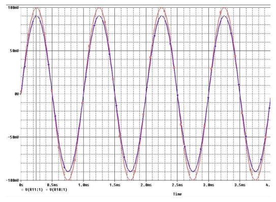
Fig. 3.8 Simulated Transient response of a first order all pass filter
