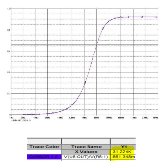
Fig 3.6 Frequency response of first order high pass filter
