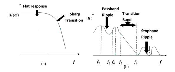
Fig. 1.1 (a) Ideal (b) Real filter characteristics
