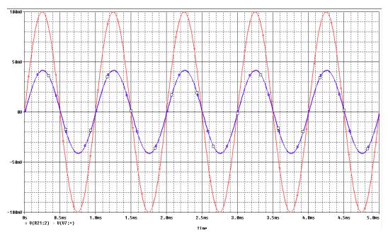
Fig 5.12 Simulating transient response of Fourth order LC low pass filter
