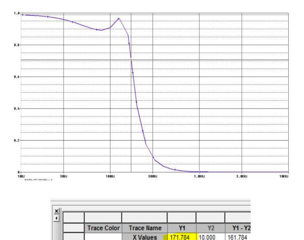
Fig 5.9 Simulated frequency response of Chebyshev third order low pass filter
