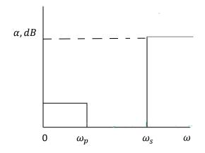
Fig 5.3 Low pass filter specification
