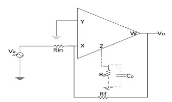
Fig 2.3 Circuit diagram of inverting amplifier
