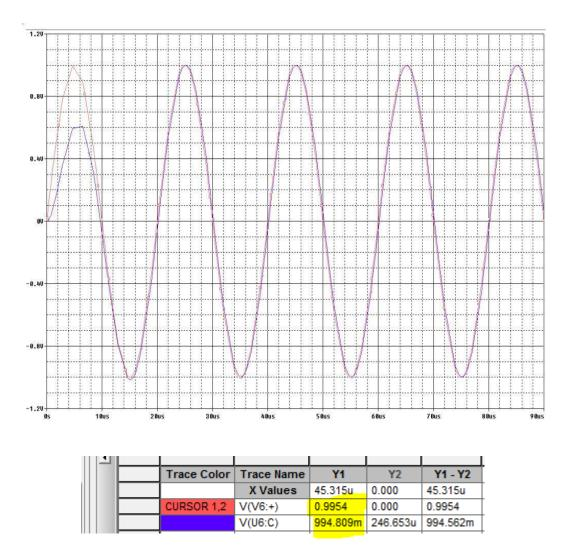
Fig 4.21 Transient response of the GIC derived band pass filter at cutoff
