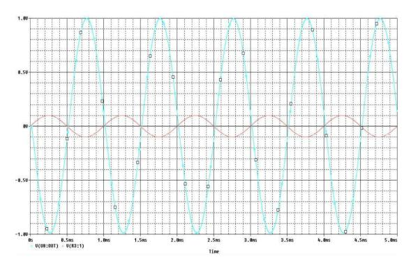
Fig 4.13 Transient response of Tow Thomas Biquad implementing inverting low pass filter.
