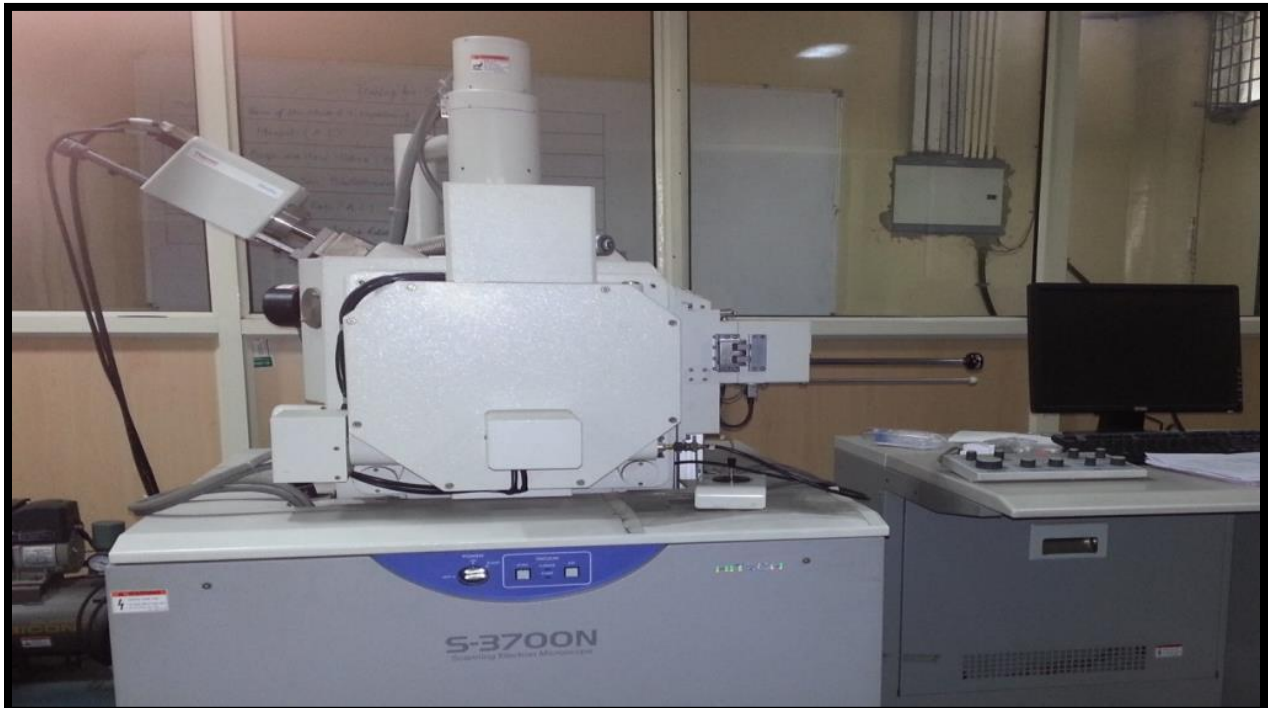
Figure 3.5: Scanning electron microscope (Hitachi S-3700N, Japan)
