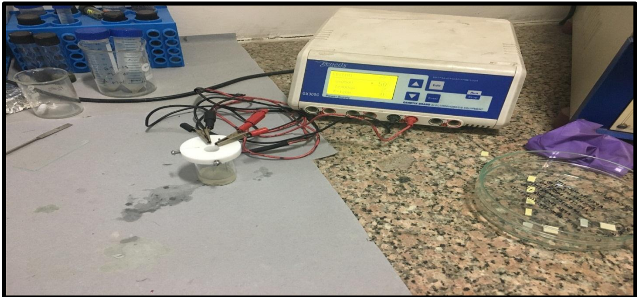
Figure 3.10: Electrophoretic deposition of /APTESFe-MoO 3 nanocomposite onto pre-hydrolyzed ITO electrode
