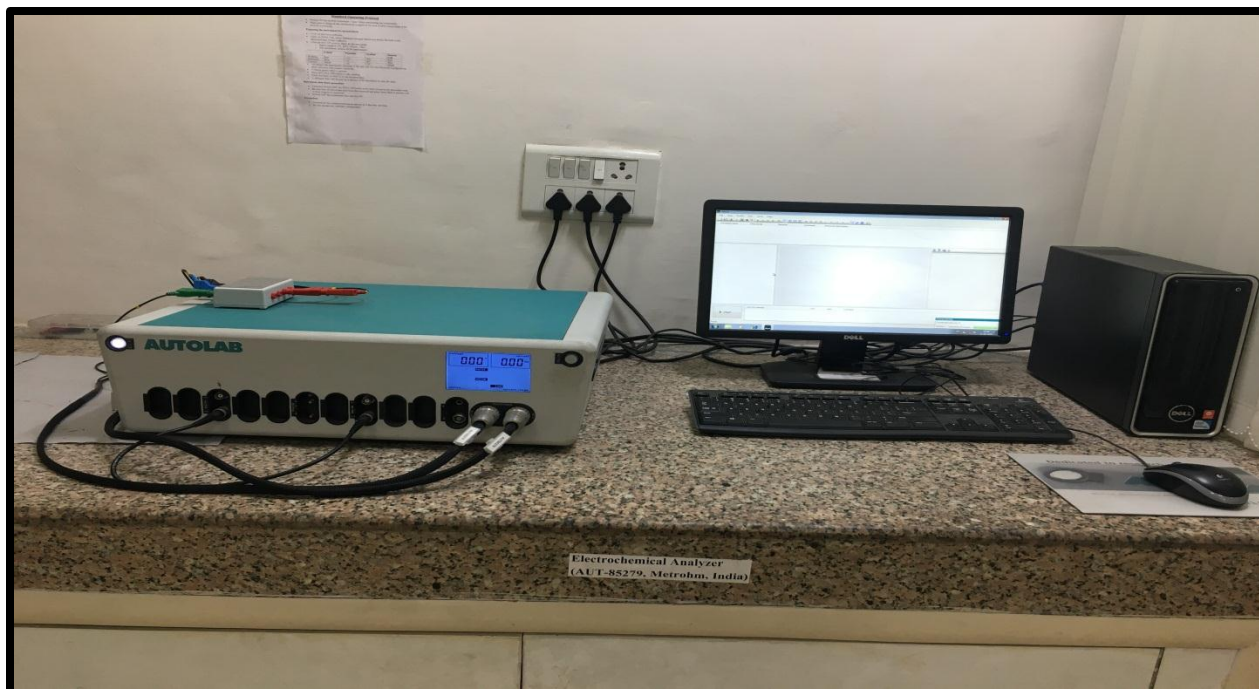
Figure 3.6: AUTOLAB, potentiostat/galvanostat ( AUT-85279, Metrohm, Switzerland).
