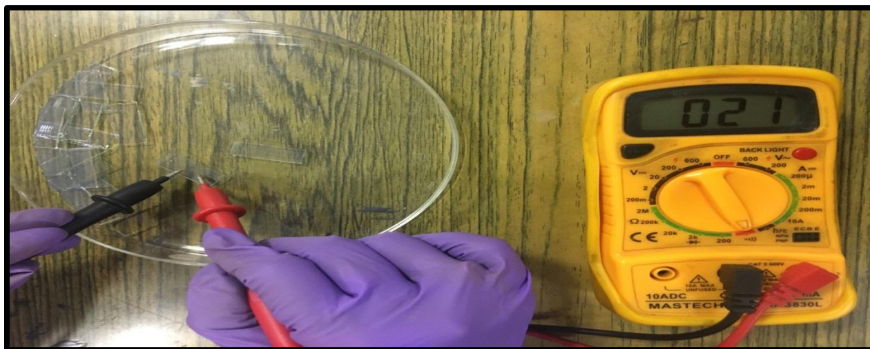
Figure 3.9: Conductivity measurement of the hydrolyzed ITO electrode
