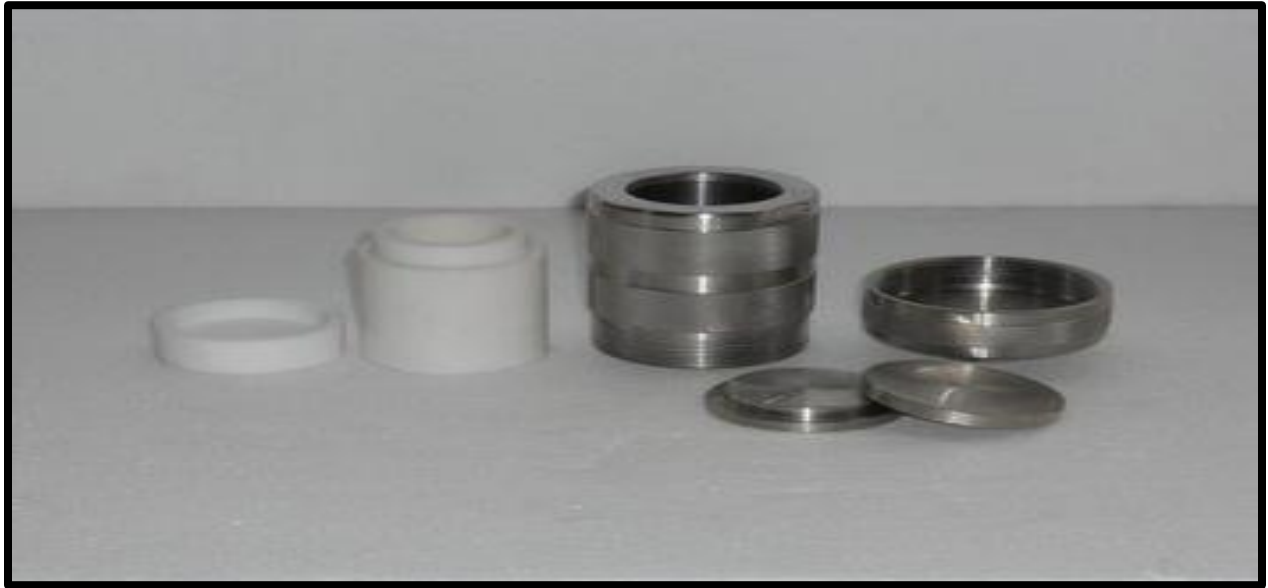
Figure 3.1: Stainless steel Teflon lined Hydrothermal vessel
