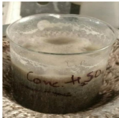
Figure 3.3 : Conc. Acid added to sand.
