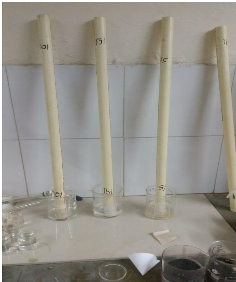
Figure 3.4 : PVC pipes filled with different % sand filtering water
