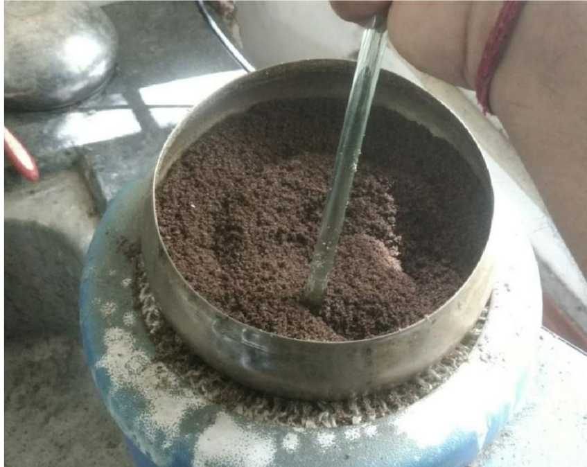
Figure 3.2 : Cooking of sand with sugar solution on heater.
