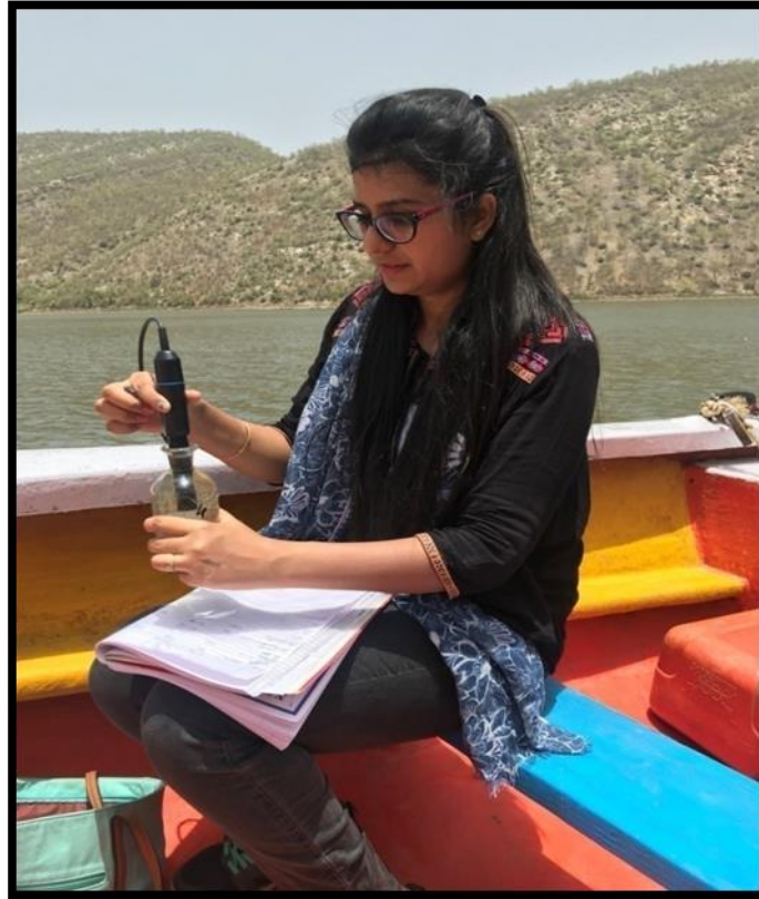
Fig 3.5 On site analysis of DO using multi-parameter meter
