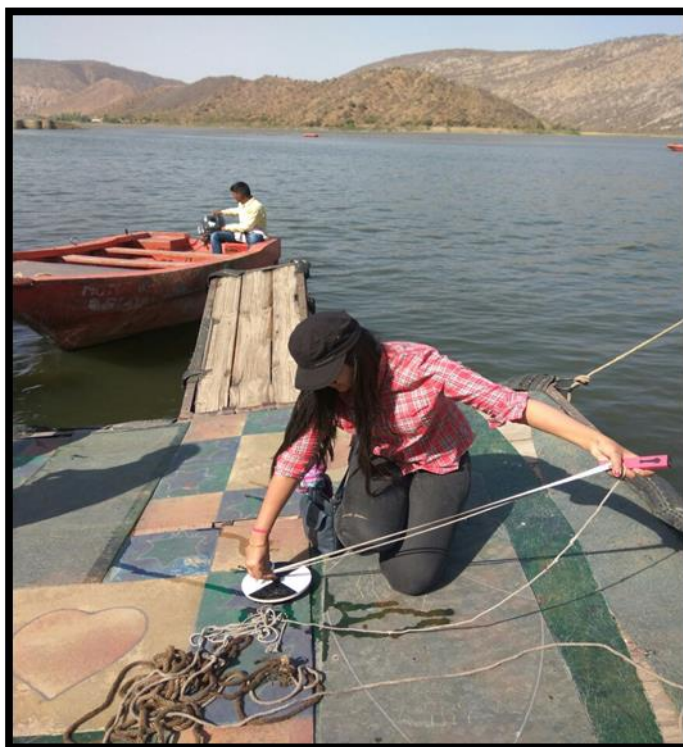
Fig 3.4 Measurement of secchi depth using secchi disc.
