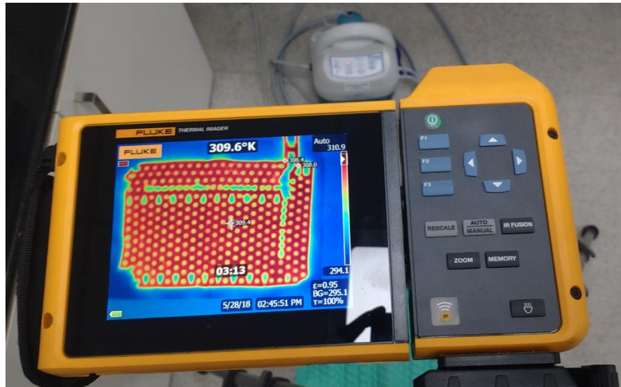
Figure 5.42 Experimental setup of thermal camera and pad
