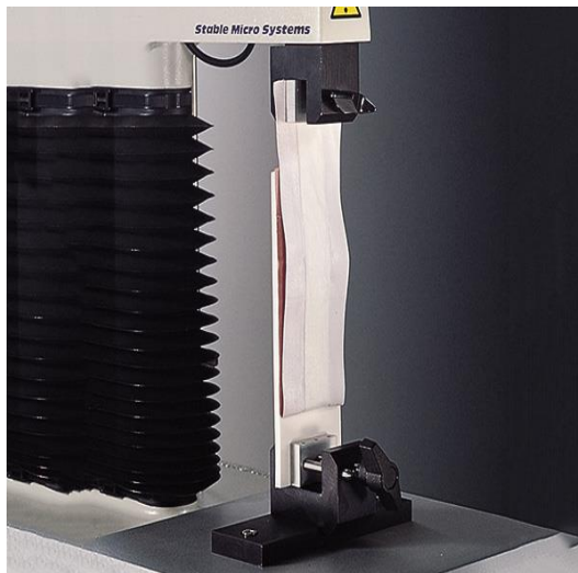
Fig. 3.7 UTM – Stable Micro Systems: TA-HD Plus Texture Analyser for peel strength analysis
