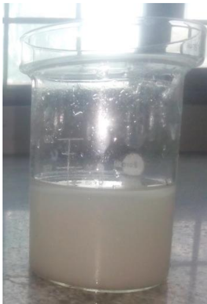
Figure 7: (a) Delignified cellulose, (b) Acid hydrolysis of delignified cellulose and (c) colloidal dispersion of acid treated cellulose
