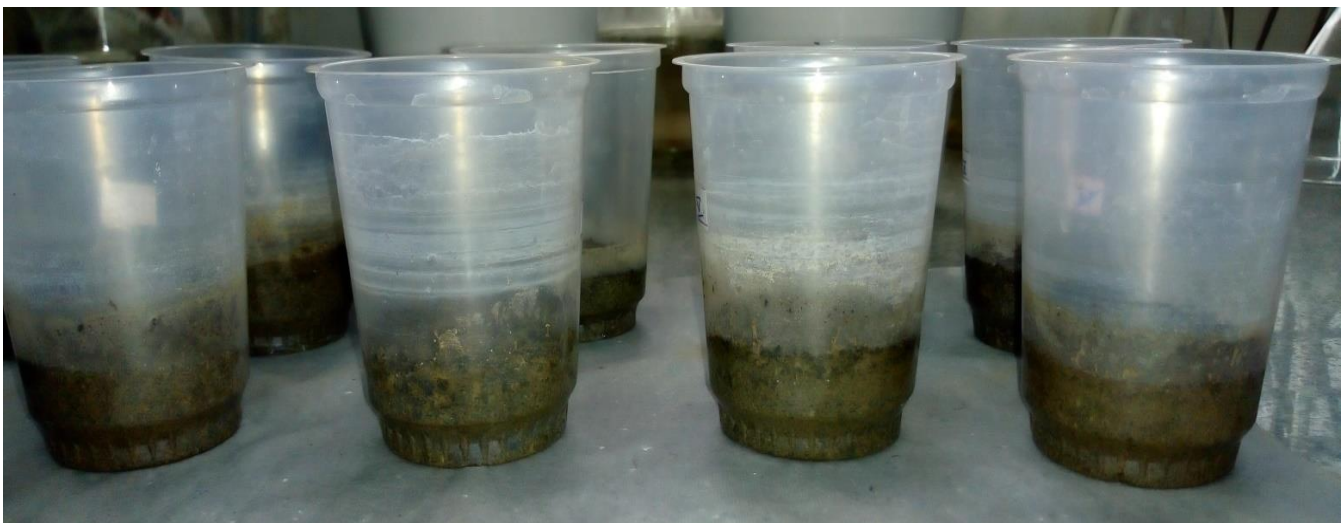
Figure 19:- Soil burial test in plastic cups containing film samples buried in soil
