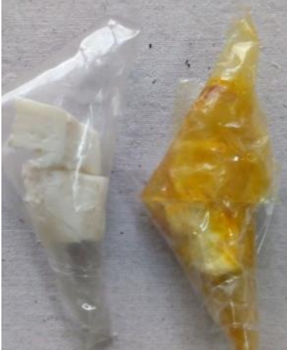
Figure 24: Cones of film samples prepared for packing of paneer.
