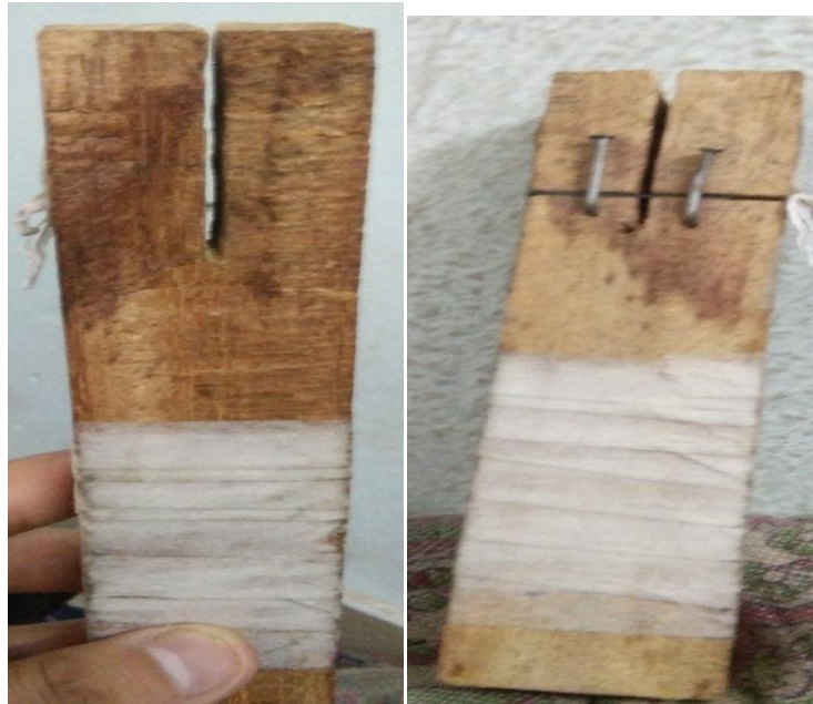
Figure 3.3 plastic bottle cutter
