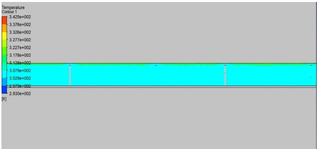
Figure 6.9: Contours of temperature at outlet at Re=790
