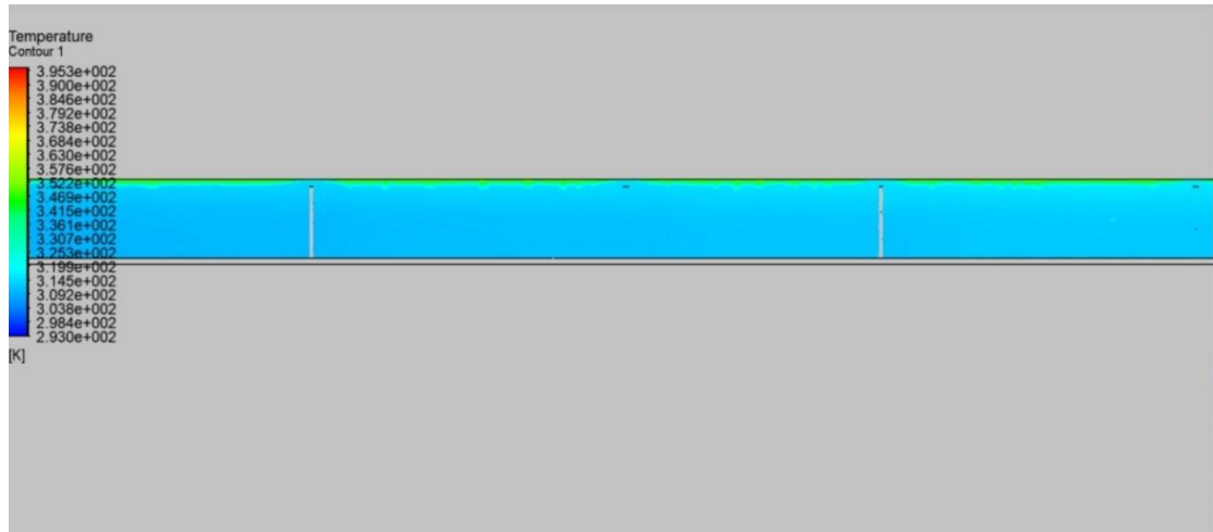
Figure 6.60: Contours of temperature at outlet at Re=1190
