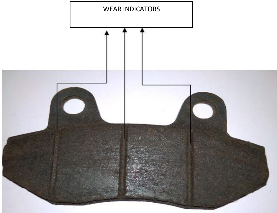
Fig. 1.10 Pad used in motorbike with wear indicators
