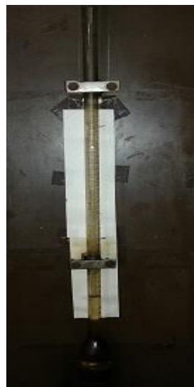
Figure 14: Fuel Flow Measuring System
