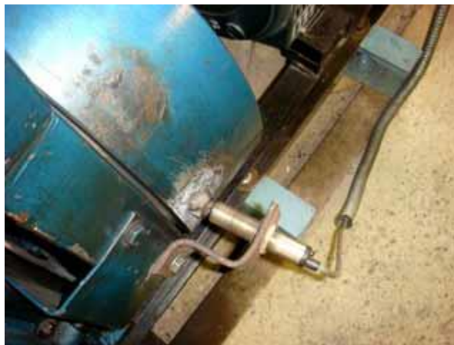
Figure15: Engine Speed Measurement
