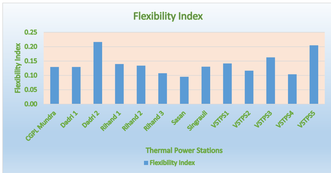
Fig. 5.2: Comparison of flexibility index for different power plants
