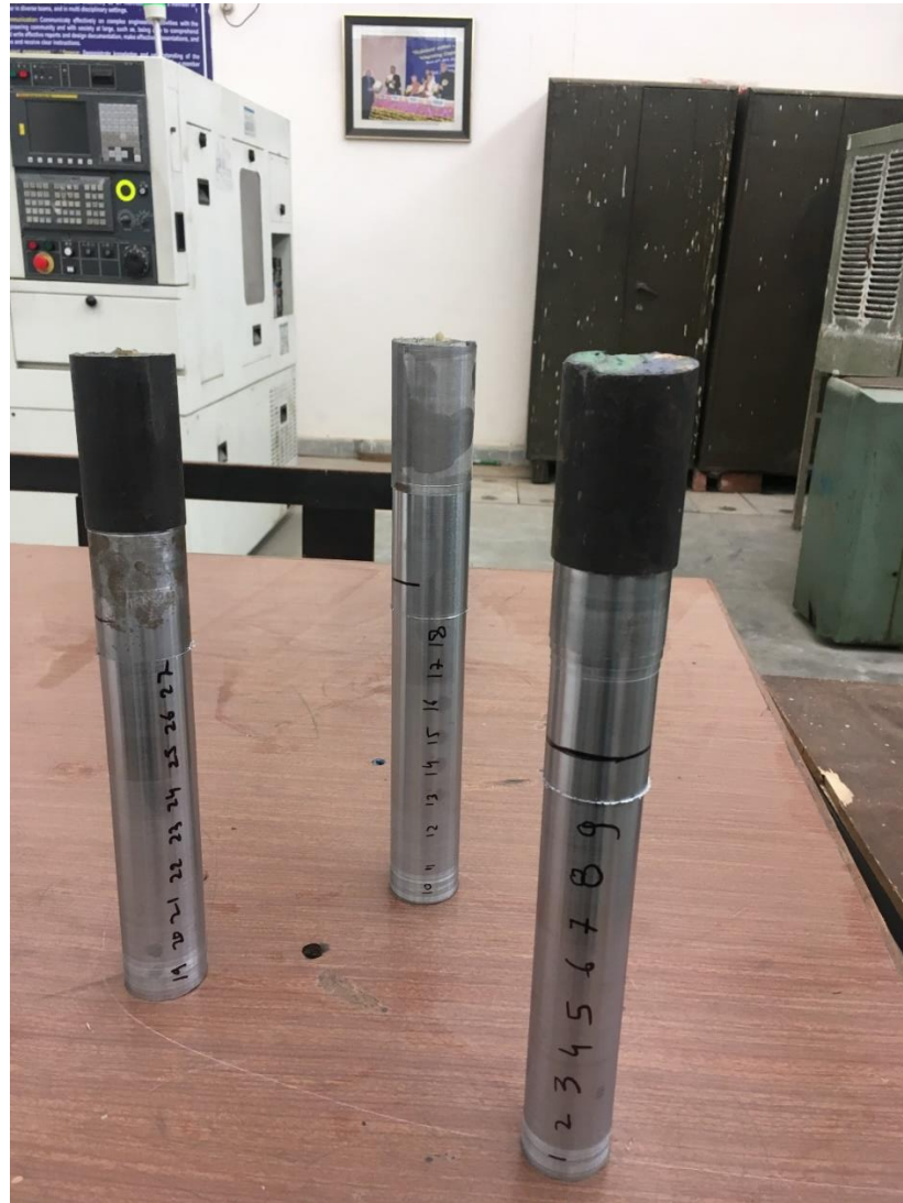
Fig. 3.9 Machined parts (mild steel EN-353)
