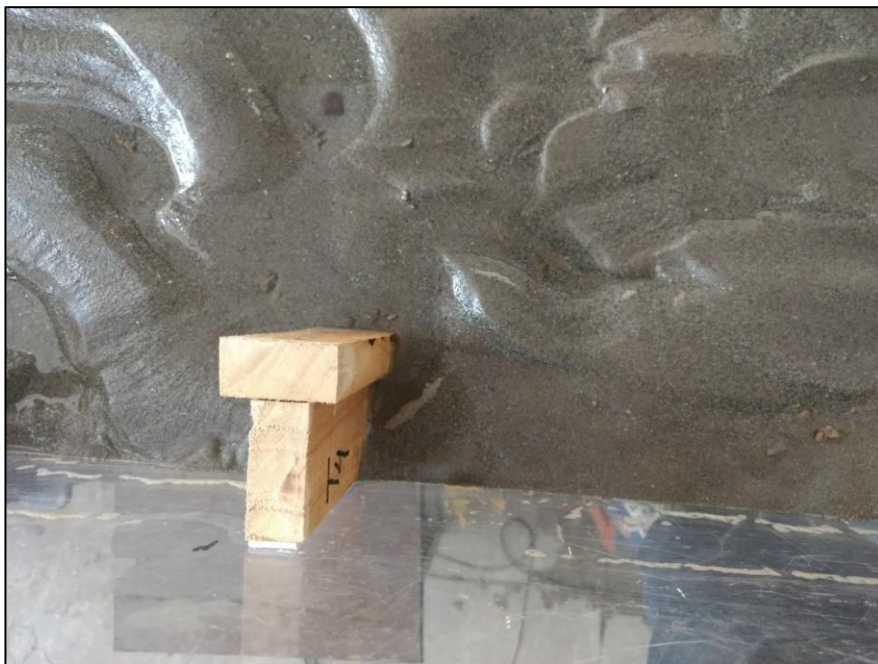
Figure.4.7 Scour formation around TG-4
