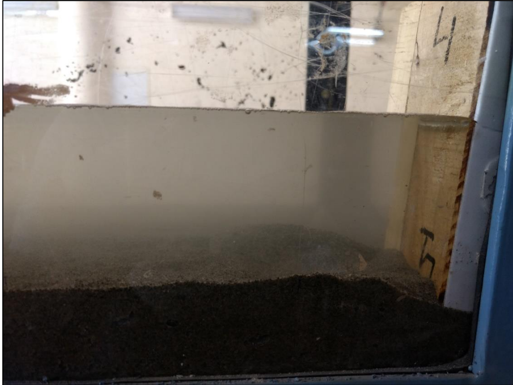
Figure.3.21 Initiation of uplift of sediment around the groynes
