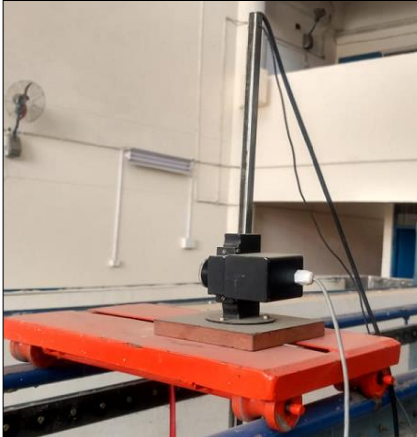
Figure.3.11 Point gauge used in the study for measurements
