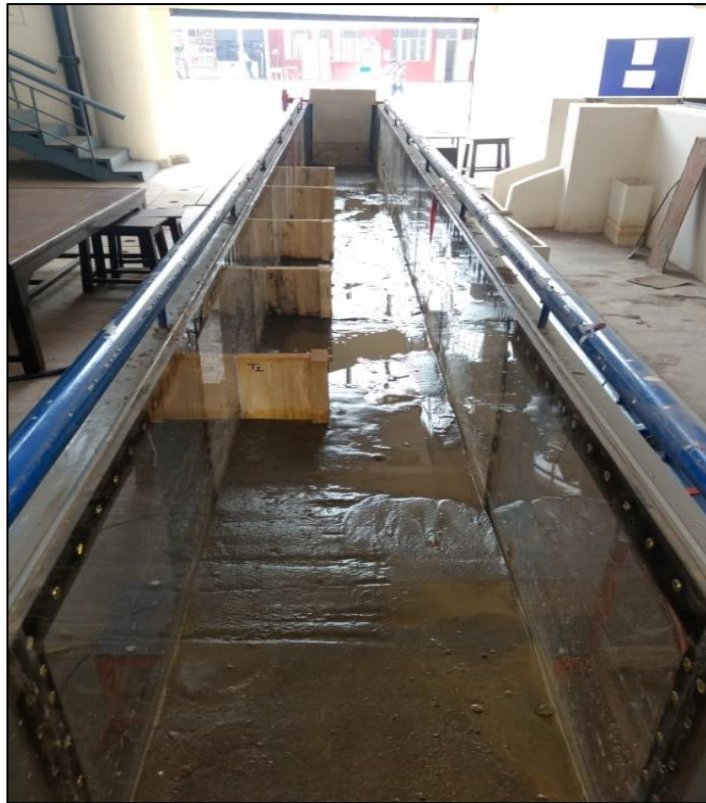
Figure.3.13 Image showing experimental setup before Test Run-1 (TG-groynes)
