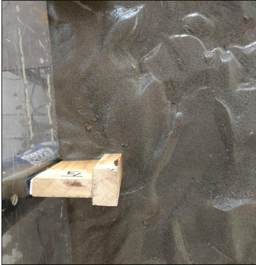
Figure.4.4 Scour formation around TG-1
