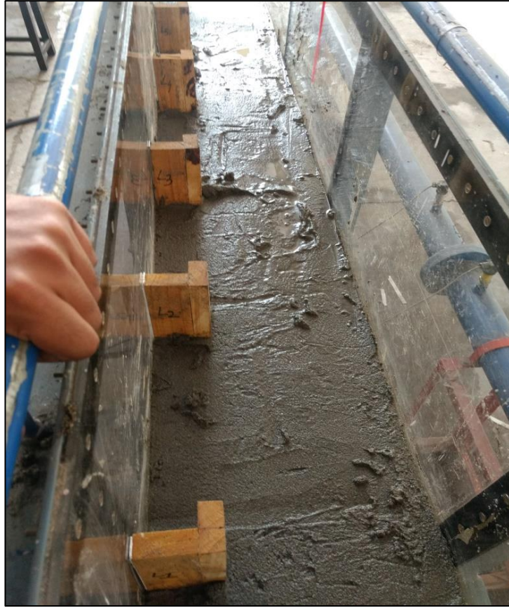
Figure.3.17 Image showing experimental setup before Test Run-3 (LD-groynes)
