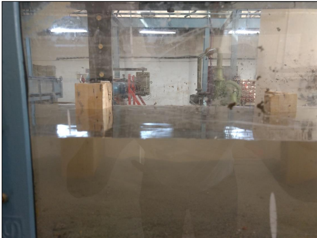
Figure.3.22 Image showing submergence of groynes during the flow
