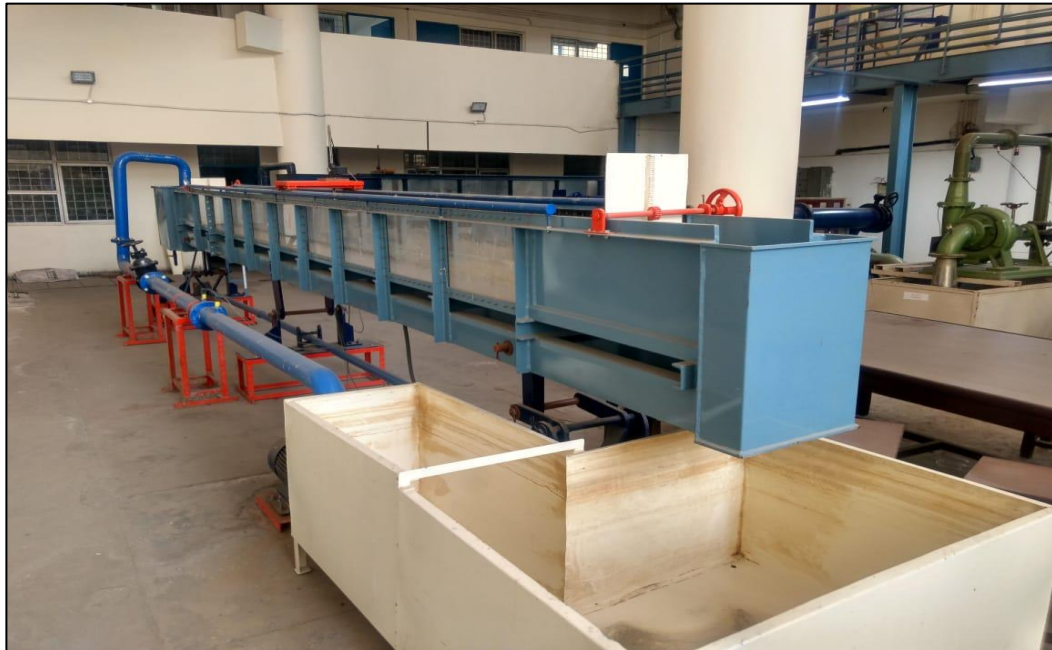
Figure.3.1 Hydraulic Flume used in the study
