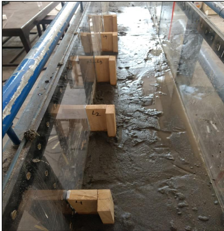
Figure.3.15 Image showing experimental setup before Test Run-2 (LU-groynes)
