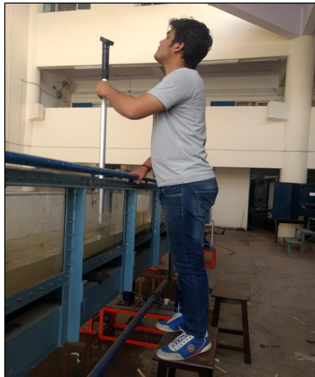
Figure.4.1 Velocity measurement using Digital Velocity Meter flow probe
