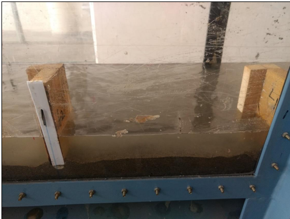
Figure.3.24 Image showing recirculation of flow in between two groynes in Test Run-3
