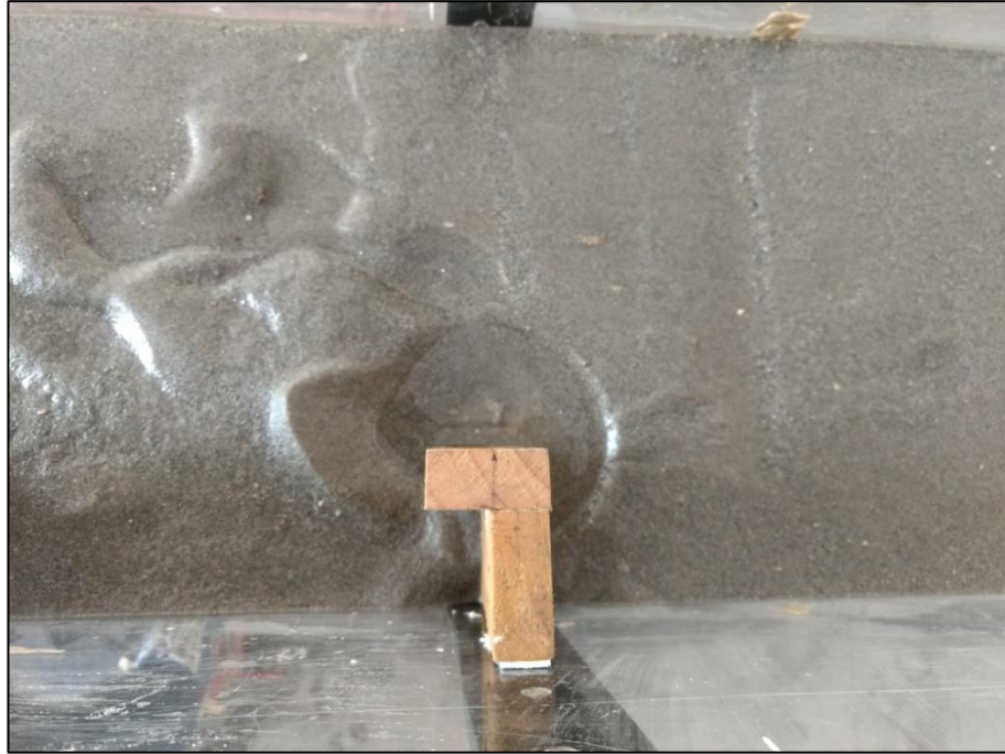
Figure.4.20 Scour formation around LD-5
