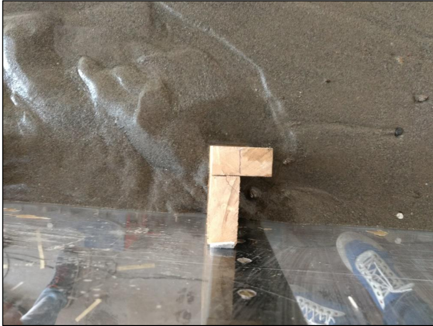
Figure.4.11 Scour formation around LU-1
