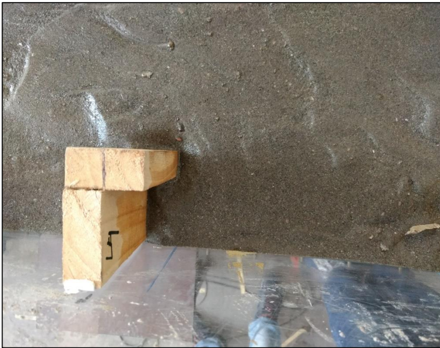
Figure.4.12 Scour formation around LU-2
