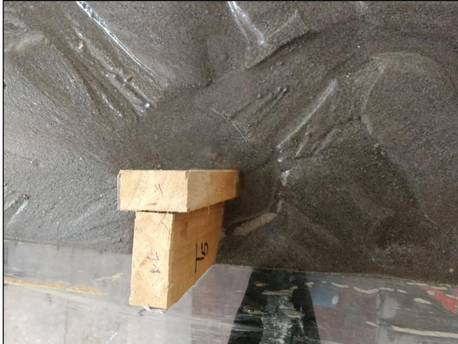
Figure.4.8 Scour formation around TG-5
