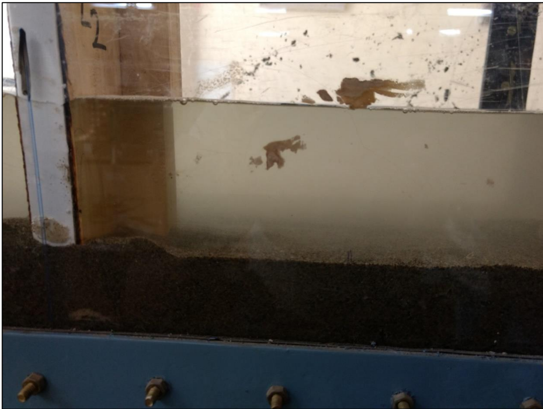
Figure. 3.20 Image showing the regime of the channel bed
