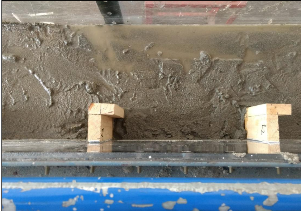
Figure.3.18 Image showing projection of groynes in Test Run-2
