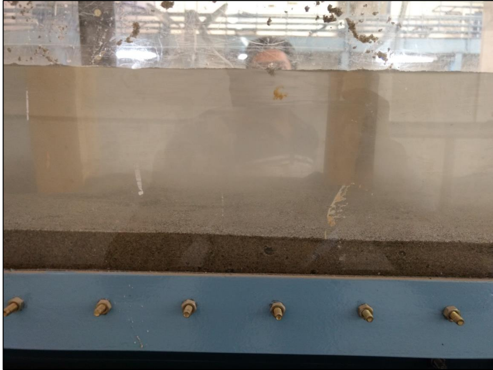
Figure.3.23 Image showing erosion of sediment in the groyne field
