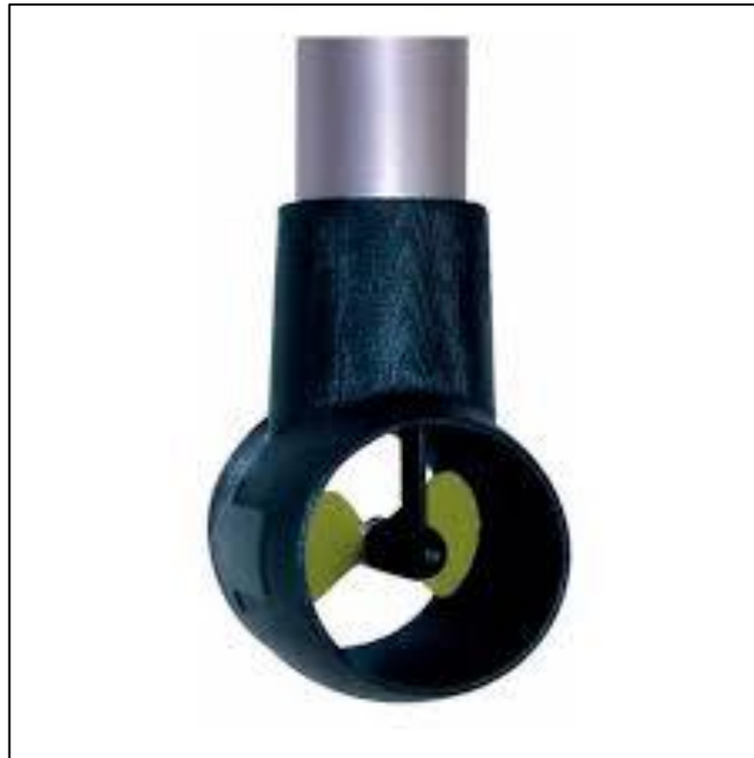
Figure.3.6 Rotating Propeller of Digital Velocity Meter (Source: Globalw.com)
