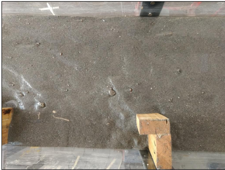
Figure.4.17 Scour formation around LD-1
