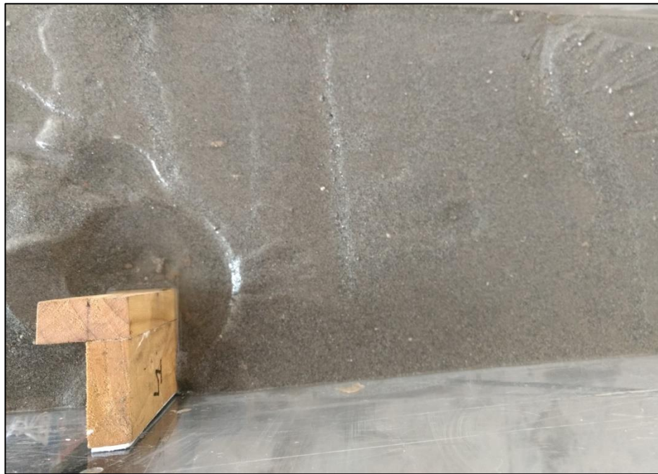
Figure.4.19 Scour formation around LD-4
