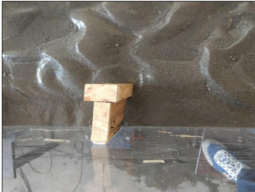
Figure.4.5 Scour formation around TG-2
