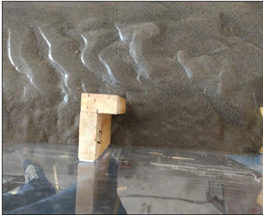
Figure.4.14 Scour formation around LU-4
