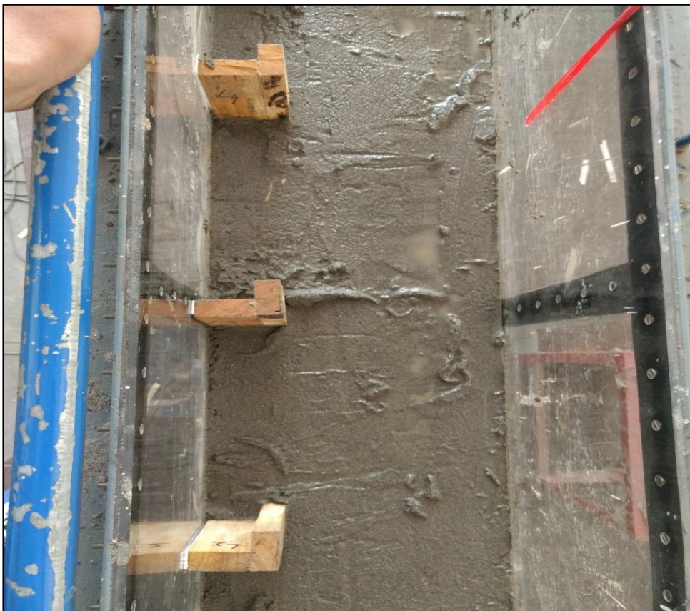
Figure.3.19 Image showing projection of groynes in Test Run-3
