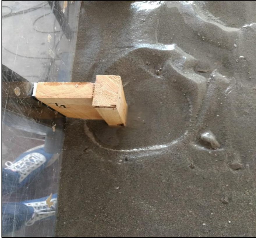
Figure.4.6 Scour formation around TG-3
