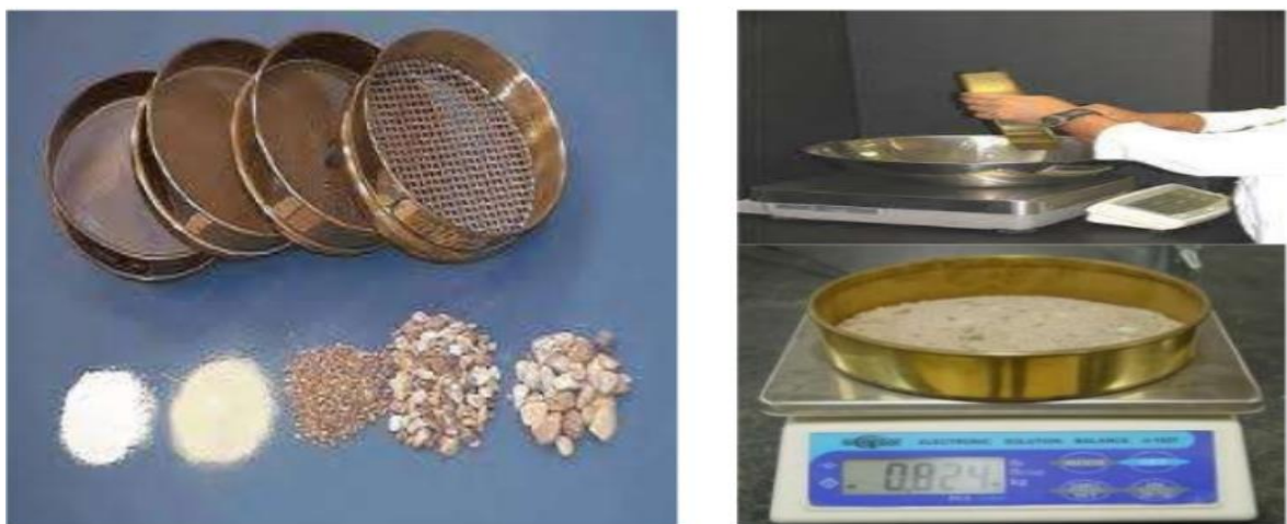
Figure 3.6: Procedure for weighing of sand (Source: Slide share uploaded by John G. Luwalaga).
