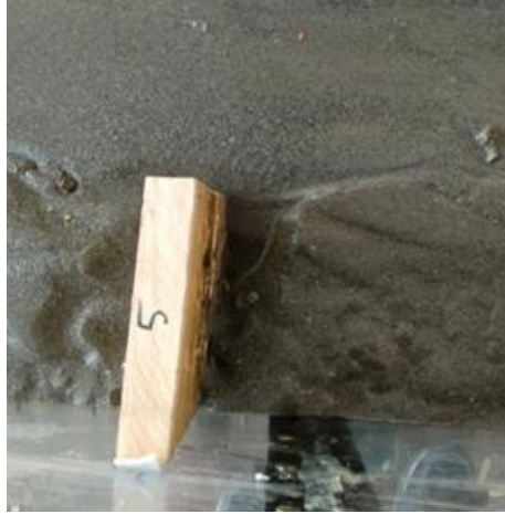
Figure 5.13.5: Scouring around fifth full length permeable groyne.
