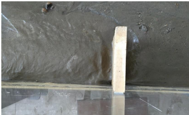
Figure 5.5.5: Scouring around fifth full length impermeable groyne.
