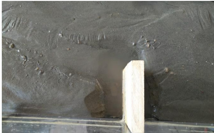
Figure 5.5.3: Scouring around third full length impermeable groyne.
