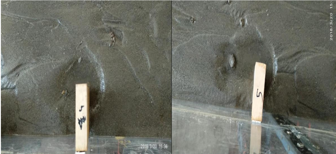
Figure 5.8.4: Scouring around fourth and fifth short length impermeable groyne.
