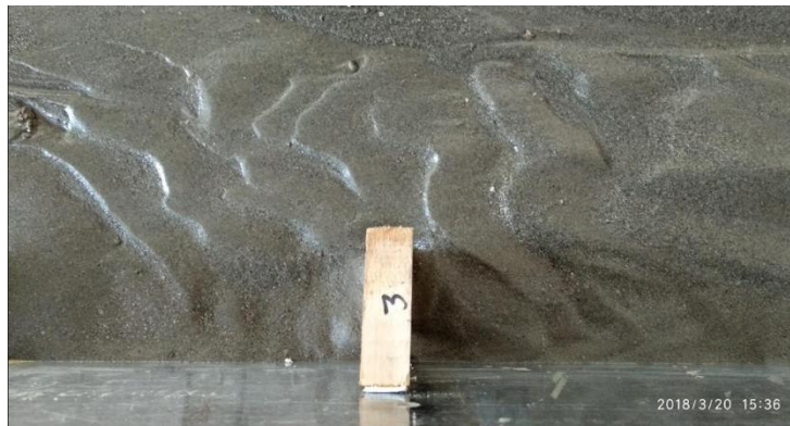
Figure 5.8.3: Scouring around third short length impermeable groyne.
