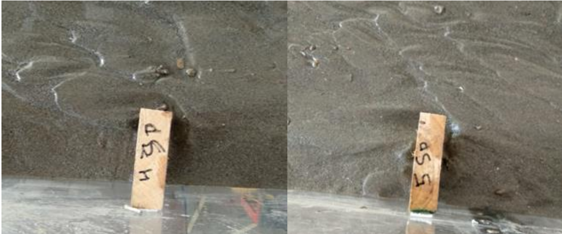
Figure 5.16.3: Scouring around fourth and fifth short length permeable groyne.
