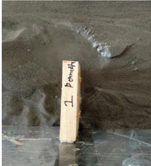
Figure 5.13.1: Scouring around first full length permeable groyne.
