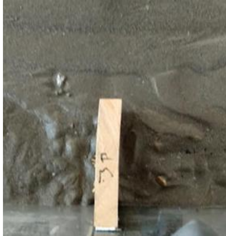
Figure 5.13.3: Scouring around third full length permeable groyne.
