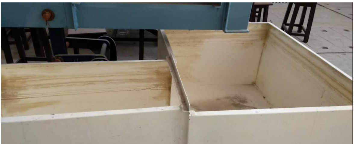
Figure 3.2: Recirculation tank attached to the tilting flume.
