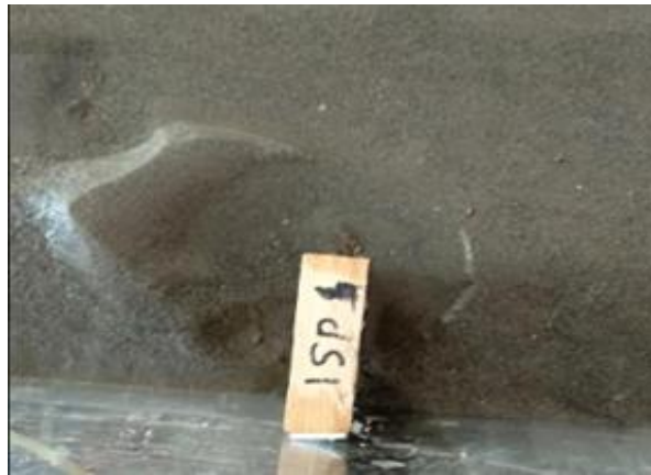
Figure 5.16.1: Scouring around first short length permeable groyne.
