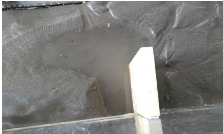
Figure 5.5.1: Scouring around first full length impermeable groyne.
