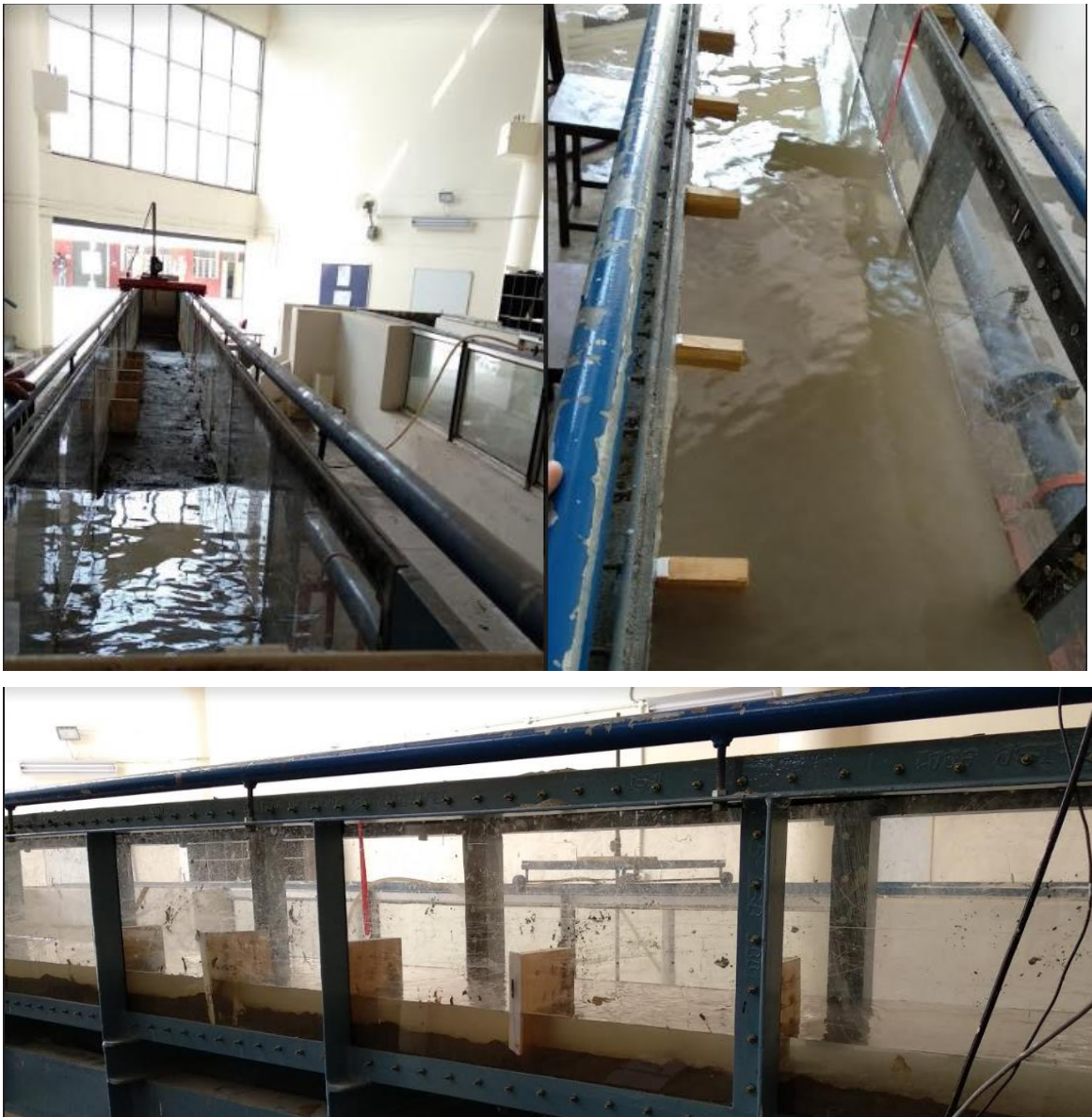
Figure 4.4: Partially submerged condition in flume during experiment.
