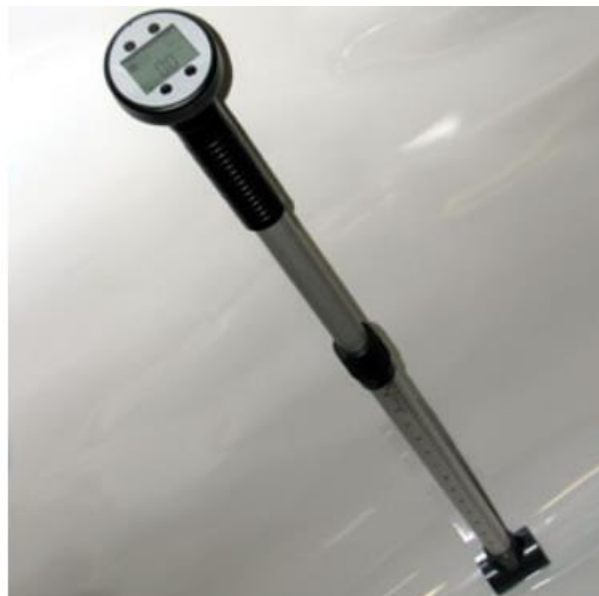
Figure 3.3: Flow probe velocity meter used for measurement of velocity (source: Global water solutions).
