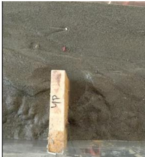
Figure 5.13.4: Scouring around fourth full length permeable groyne.
