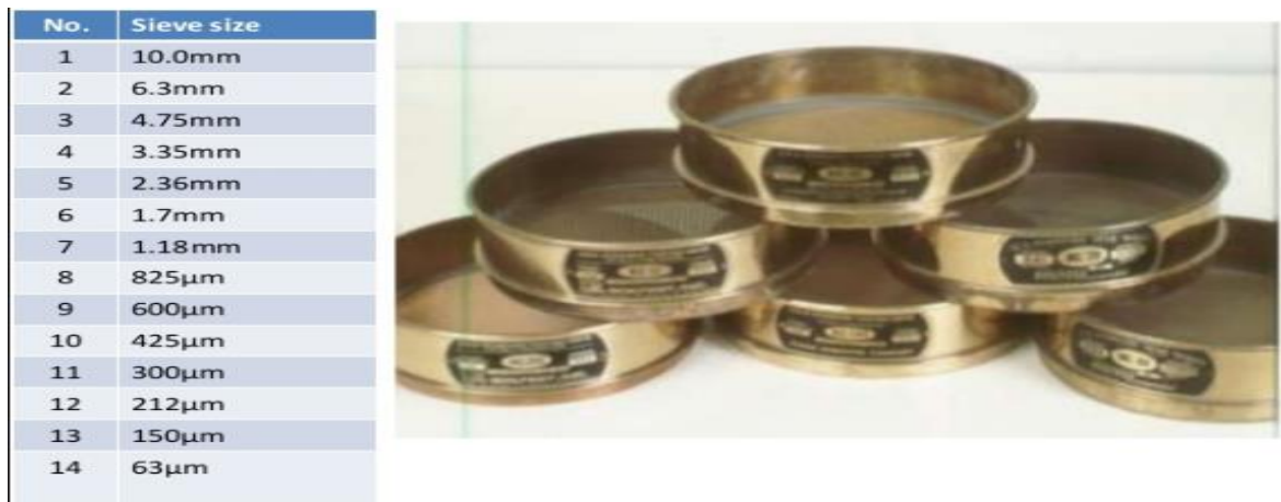
Figure 3.5: Arrangement of sieves in decreasing order (Source: Slide share uploaded by John G. Luwalaga)
