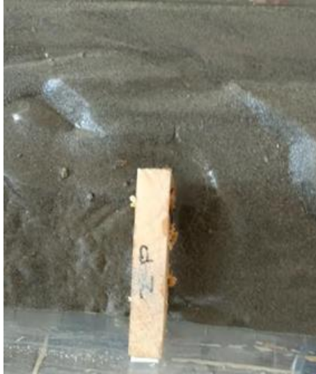
Figure 5.13.2: Scouring around second full length permeable groyne.
