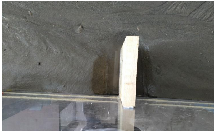
Figure 5.5.4: Scouring around fourth full length impermeable groyne.
