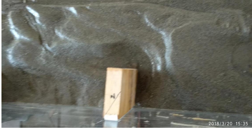
Figure 5.8.2: Scouring around second short length impermeable groyne.
