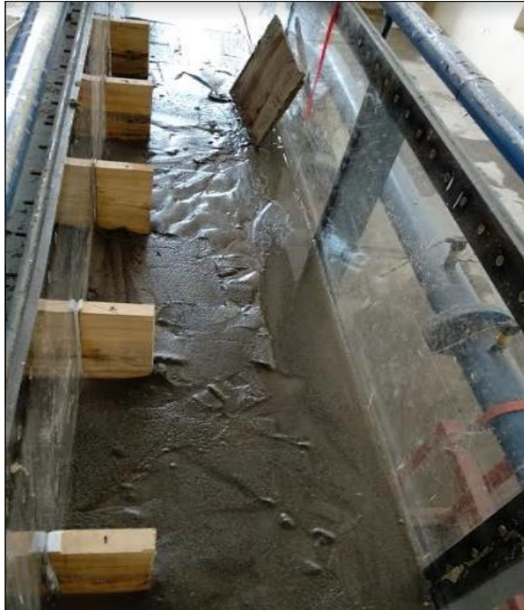
Figure 4.2: Placement of Short Impermeable groynes.
