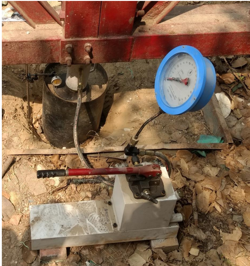
Fig 3.11 Plate load test
