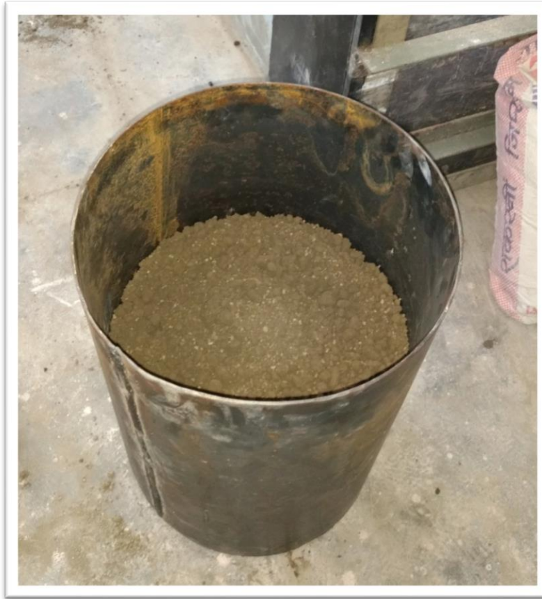
Fig.3.3. M.S steel circular tank of dia. 65cm
