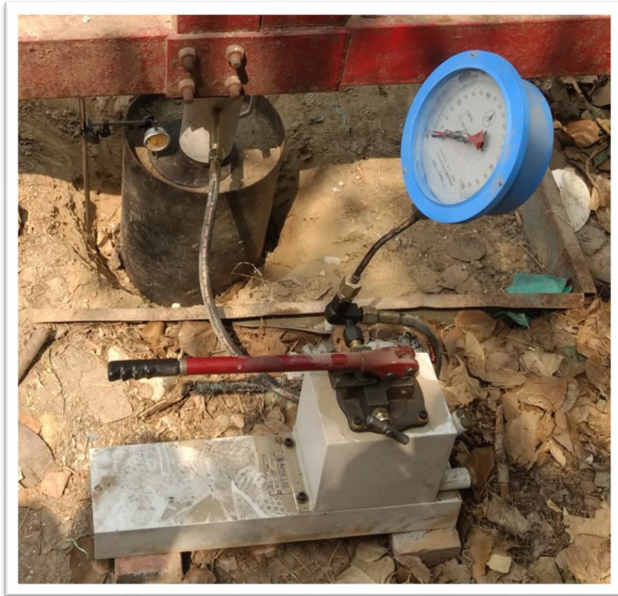
Fig 3.6 Hydraulic jack and Test setup
