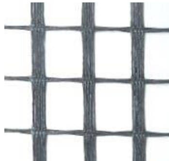
Figure 1.3 Geogrid sample manufactured by knitting (Courtesy: The Constructors: Civil Engineering Home for Civil Engineers)
