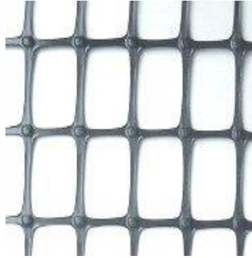
Figure 1.2 Geogrid sample manufactured by Extruding (Courtesy: The Constructors: Civil Engineering Home for Civil Engineers)
